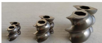
Figure 1. The three scales in this study: 11 mm, 16 mm and 24 mm sized twin-screws.
