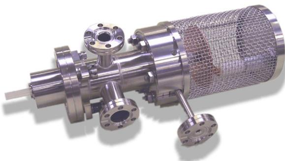
Figure 17. Discharge lamp used for UPS.
