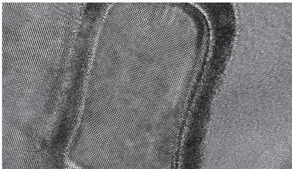
An atomic resolution image of an advanced logic semiconductor device is depicted. Some of the layers critical to chip performance are only a few atoms in width.
