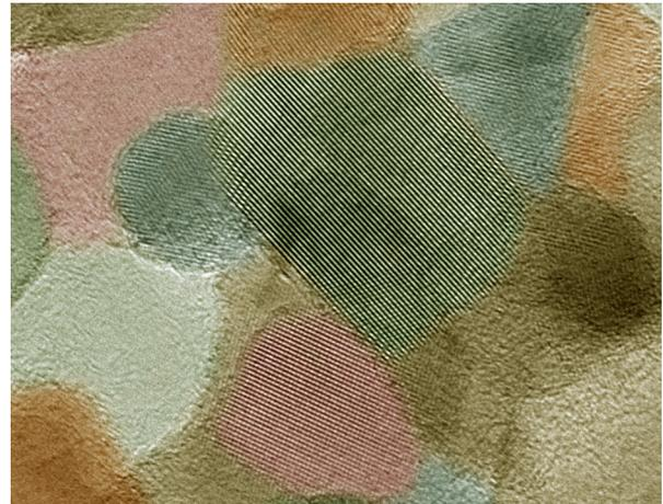
This image displays the formation of planes that are visible when nanoparticles of titanium dioxide are used as a catalyst in the process of photocatalysis.
