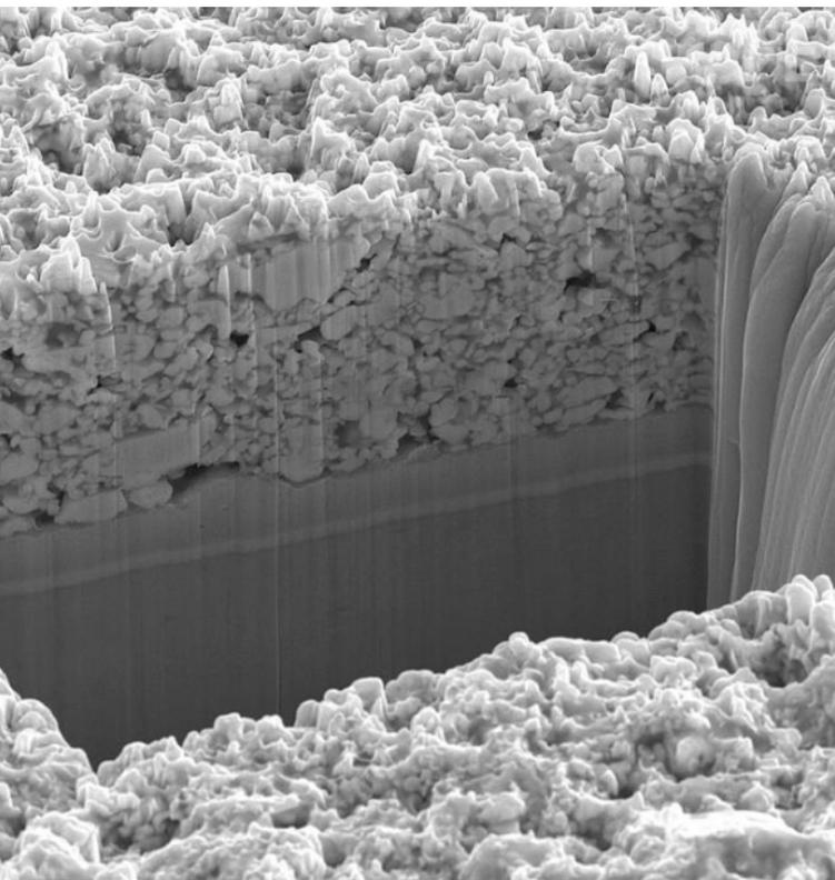
Cross-section made by FIB milling of a multilayer photovoltaic panel.
