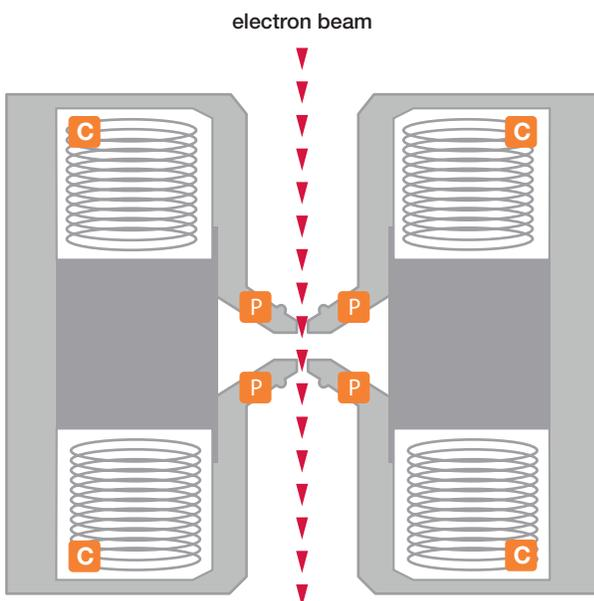
Cross-section of an electromagnetic lens.
