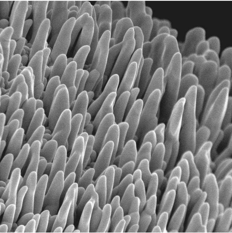
Platinum nano-features fabricated by FIB microscopy and imaged using SEM.
