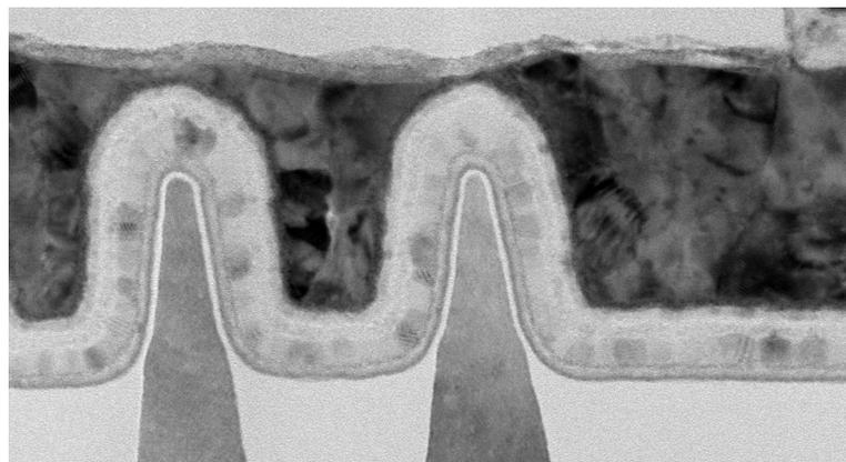
Bright Field TEM of a 3D transistor used in microprocessors. The gate of the transistor is wrapped around the source drain to increase performance.
