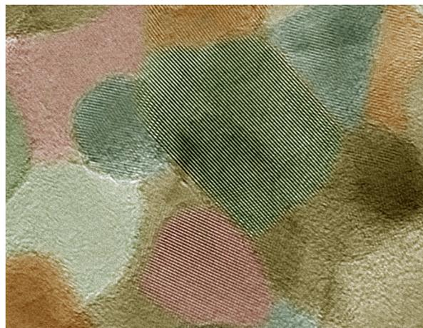
This image displays the formation of planes that are visible when nanoparticles of titanium dioxide are used as a catalyst in the process of photocatalysis.
