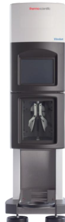
Automated systems, like the Thermo Scientific™ Vitrobot™ System, provide fast, easy and reproducible sample preparation.
