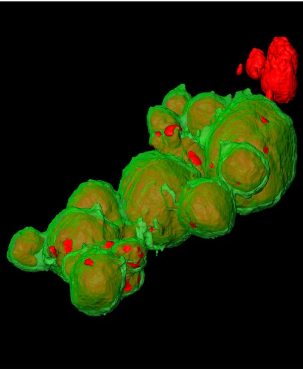
3D EDS tomogram of Ag-Pt core-shell nanoparticles, where most of the Ag cores (red) are covered by Pt shells (green). Pores in the Pt partially expose the cores.
