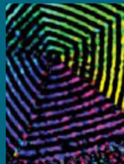
Moiré-fringe image extracted from the original TEM image taken on a spherical-aberration corrected S/TEM.
