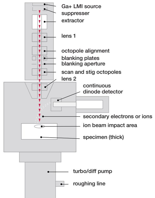
Components of a FIB microscope.
