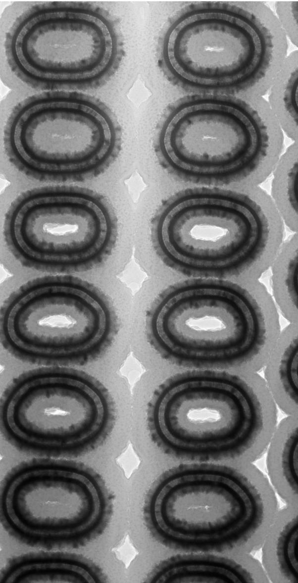
Dynamic random-access memory (DRAM) capacitors, a type of random-access memory that stores each bit of data in a separate capacitor within an integrated circuit.
