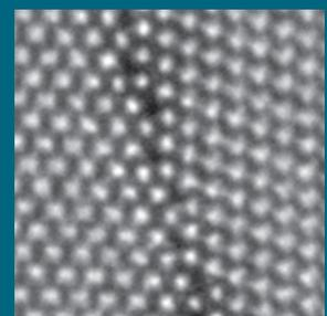
Comparison of HR-TEMs with (left) and without (right)  $C_s$ -correction on the same Si (110) grain boundary at 300 kV.
