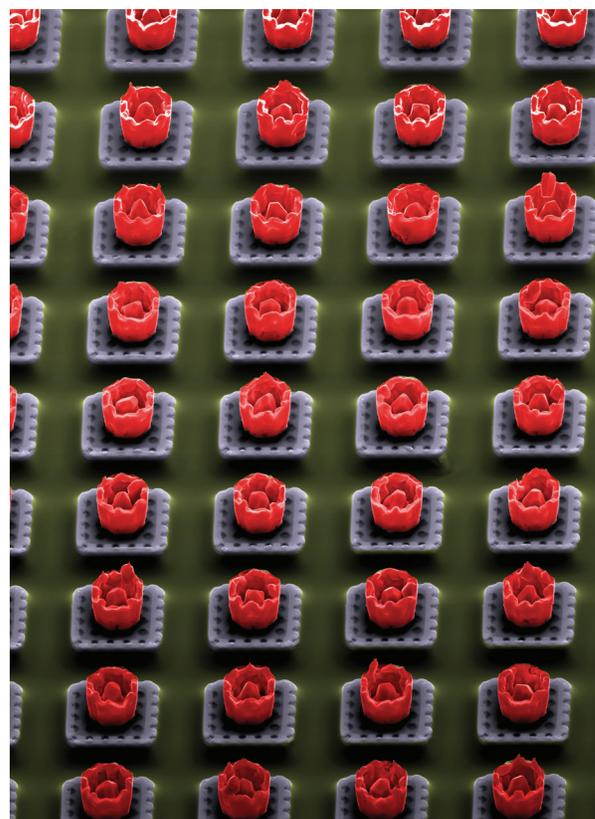
Contact side of an infrared detector array.
