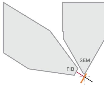
Diagram illustrating the DualBeam system, a combined application of a focused ion beam (FIB) and SEM on a sample (orange).
