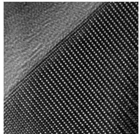
Hematite nanoparticle with individual atoms visible.
