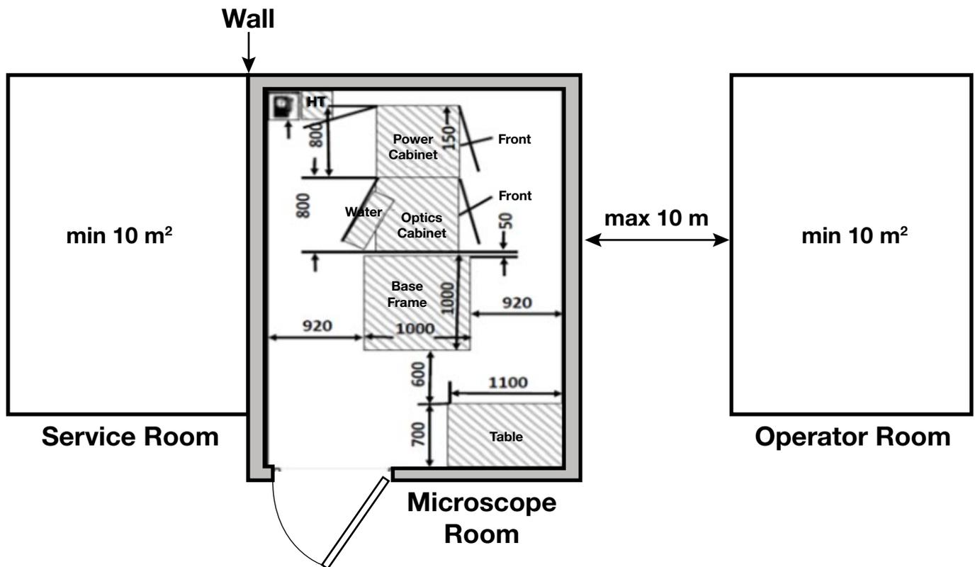
Figure 3. Recommended room layout for Talos L120C. The indicated dimensions are in millimeters.
