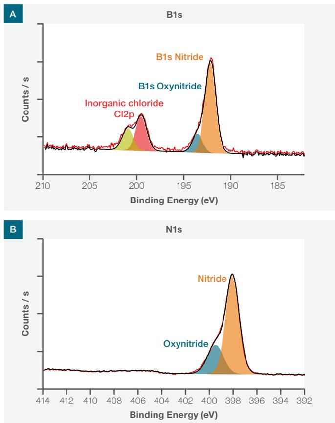
Figure 3: High-resolution deconvoluted XPS spectra of B1s (a) and N1s (b) taken at point P1 showing different chemical states.
