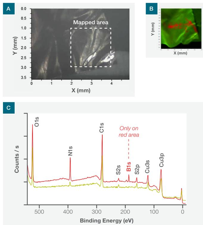
Figure 2: (a) Optical image of the sample from one of the three Nexsa Surface Analysis System cameras, (b) N1s nitride XPS SnapMap image of the mapped area and (c) XPS survey spectra at the points P1 and P2 shown in (b).
