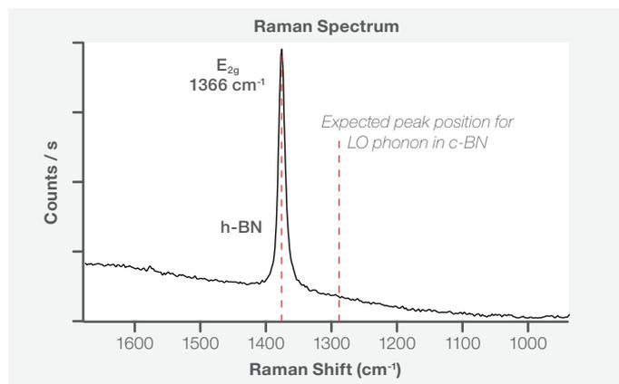
Figure 4: Raman spectra at point P1 using 532 nm laser line.
