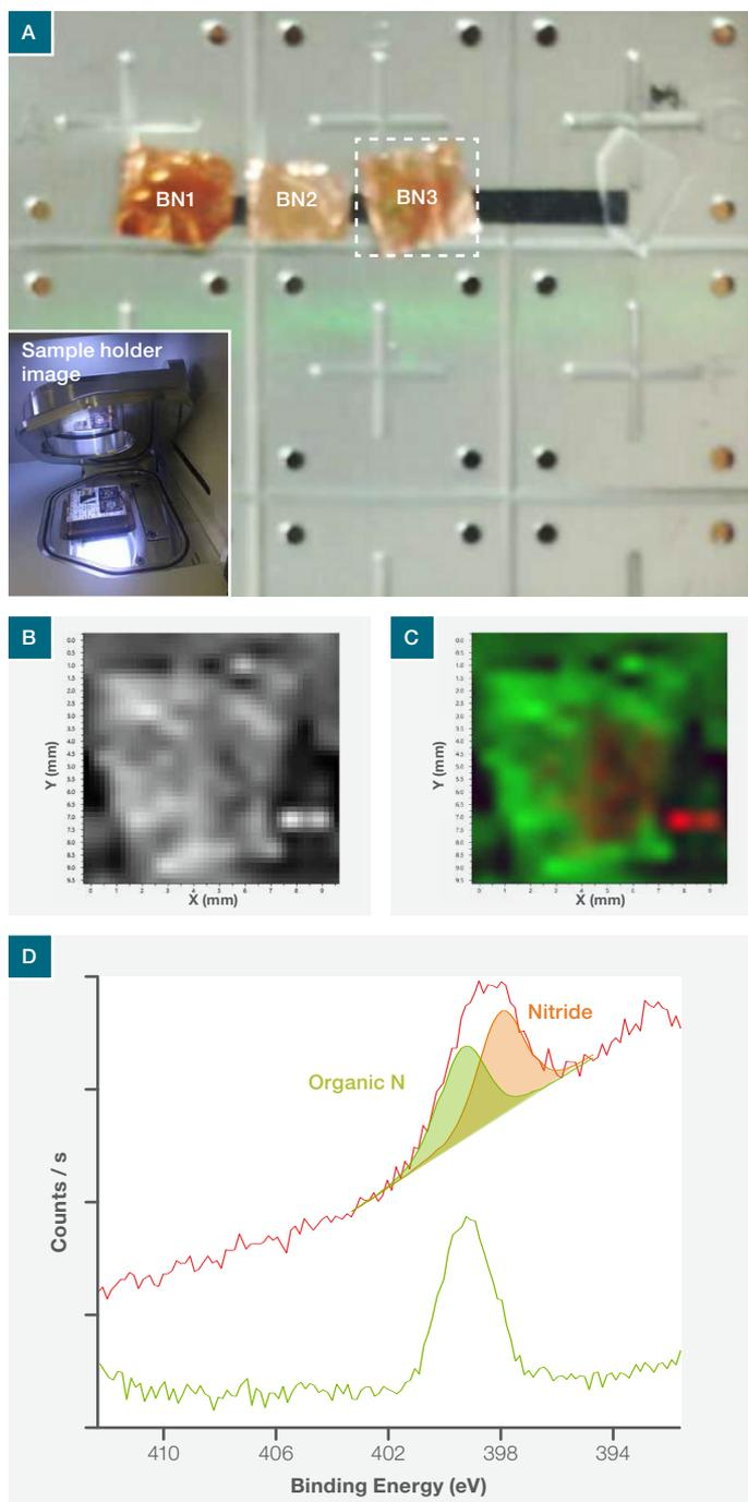
Figure 1: (a) Nexsa Surface Analysis System optical image of the whole sample platter (inset shows the sample holder in loading position), (b) N1s intensity map across whole of the sample (c) chemical state N1s intensity map and (d) N1s average spectra from the green and red regions on map.
