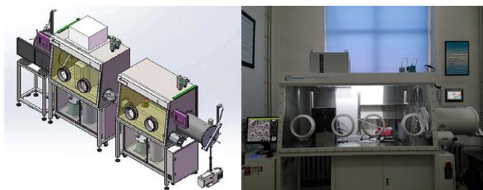
Figure 1. Left: schematic of workflow incorporating a Phenom XL G2 Desktop SEM inside a glove box. Right: actual setup of Phenom Desktop SEM inside argon filled glove box.
