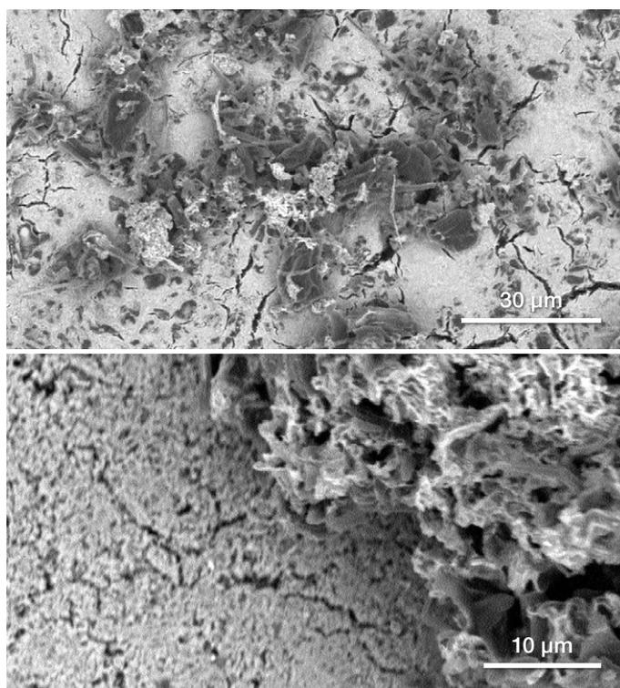
Figure 3. SEM images of lithium dendrites acquired with Phenom SEM inside argon filled glove box. The image below displays the script Ultra Depth of Focus, providing a cross-section sample of an anode.
