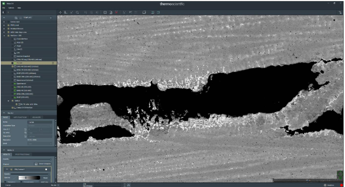
Figure 3. High-resolution BSE image of fracture along grain boundaries within the Inconel coupon. High concentration of dendritic melt phases indicates improper build conditions leading to an unstable microstructure during cooling of the build. BSE imagery was used to select locations for EBSD analysis.
