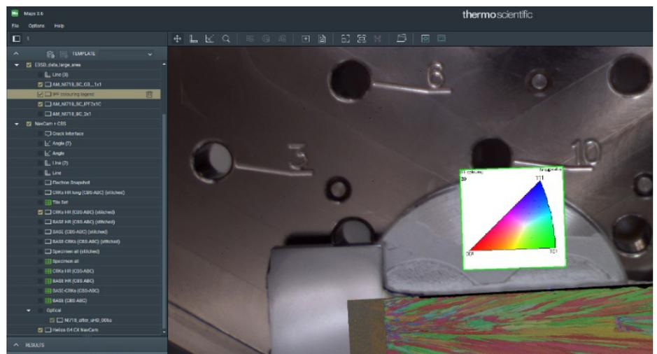
Figure 4. Tiled EBSD map of full sample overlaid on Nav-Cam Camera background image. Inverse Pole Figure image is also placed directly in Maps Software. Each layer can be turned on or off as the use requires for visualization. EBSD map shows crystallographic orientation of large columnar grains.
