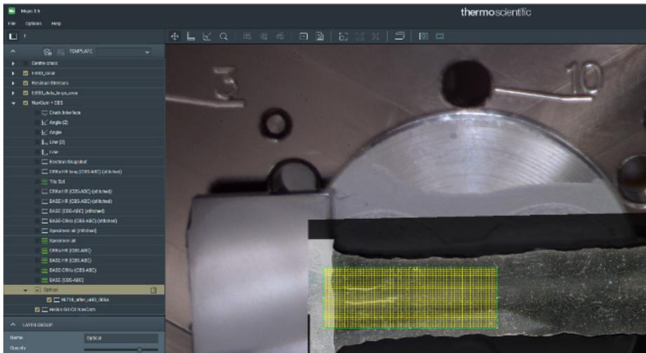
Figure 2. Maps Software UI illustrating the Nav-Cam Camera image background with over-layed optical image and tileset (yellow grid) that is the target for high-resolution BSE image acquisition.
