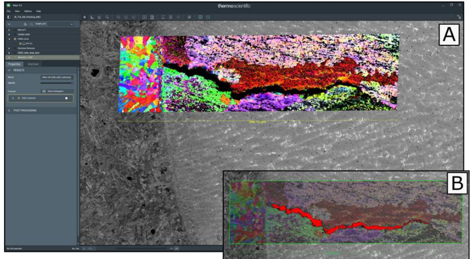
Figure 5. A) BSE image background with an EBSD map around a fractured region of the Inconel coupon. B) Same image as A, illustrating transparency of EBSD map on the BSE background image. Maps Software also provides the ability to threshold an image to highlight specific features. In this case, illustrating the difference in fracture aperture captured in EBSD versus BSE imagery.
