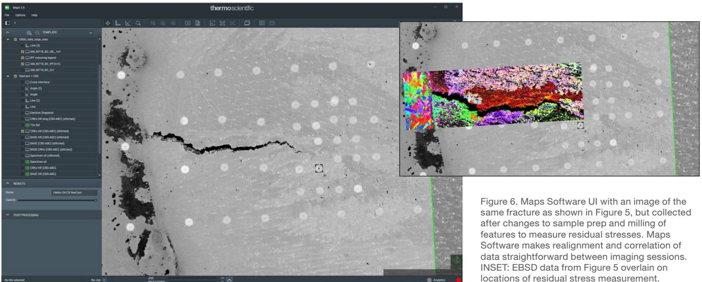
Figure 6. Maps Software UI with an image of the same fracture as shown in Figure 5, but collected after changes to sample prep and milling of features to measure residual stresses. Maps Software makes realignment and correlation of data straightforward between imaging sessions. INSET: EBSD data from Figure 5 overlain on locations of residual stress measurement.
