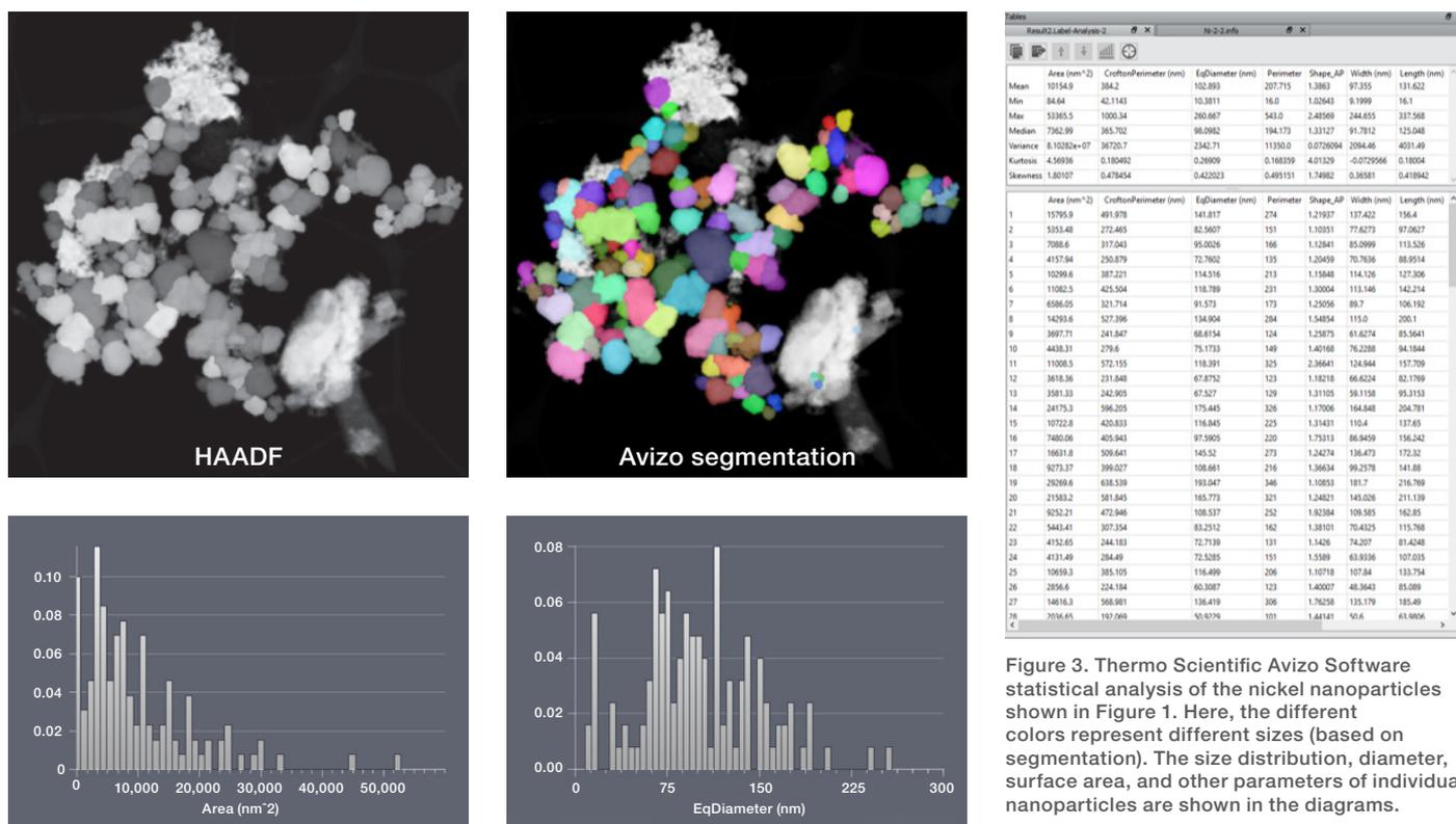
Figure 3. Thermo Scientific Avizo Software statistical analysis of the nickel nanoparticles shown in Figure 1. Here, the different colors represent different sizes (based on segmentation). The size distribution, diameter, surface area, and other parameters of individual nanoparticles are shown in the diagrams.
