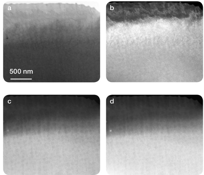
Figure 3. S/TEM images acquired simultaneously from 4 different STEM detectors: a) Bright field STEM; b) dark field STEM; c, d) high angle dark field.
