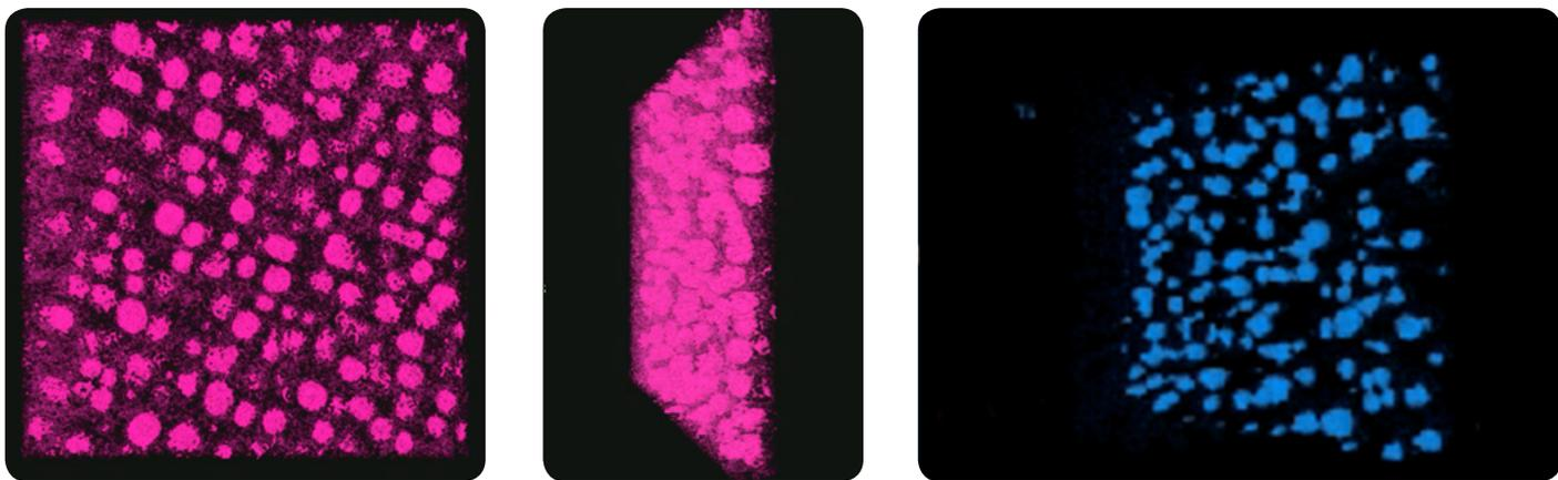
Figure 7. 2D-3D EDS maps showing spatial distribution of individual elements in super alloy lamella ( 1.2µm × 1.2µm × 0.1µm).
