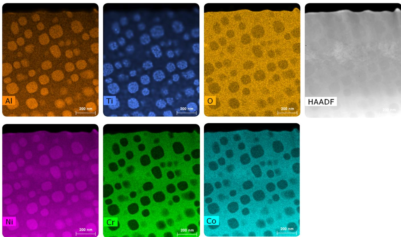
Figure 5. 2D EDS compositional maps of the elements acquired with Super-X system on Talos S/TEM. Maps of 280 × 235px were acquired and quantified in <10 minutes.
