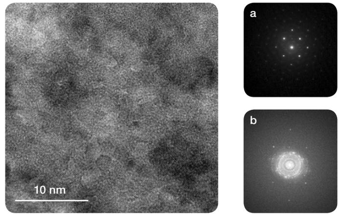
Figure 2. HR-TEM image of superalloy, 4k x 4k pixels; a) SAED diffractogram; b) FFT diffractogram from the HRTEM image.
