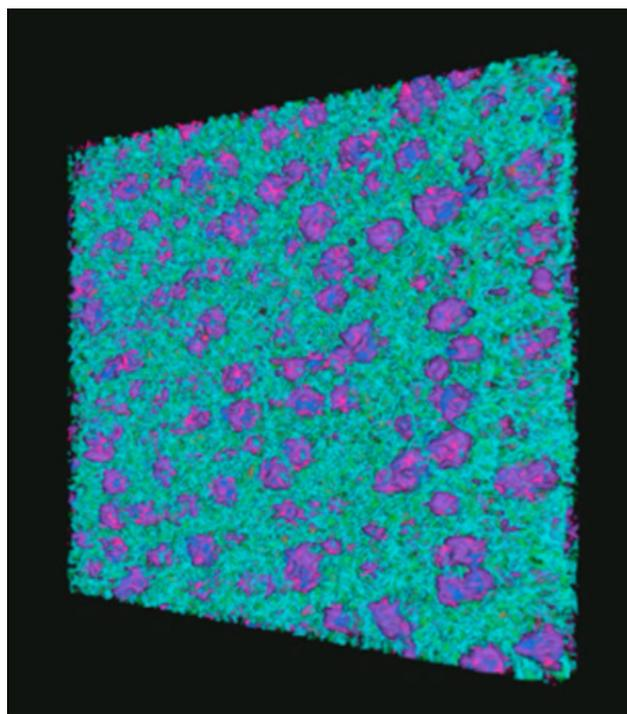
Figure. 1 b. 3D EDS multi-element compositional map, tilt range +/-70 degrees; 512 × 512 pixels at each tilt – total acquisition time <3h.
