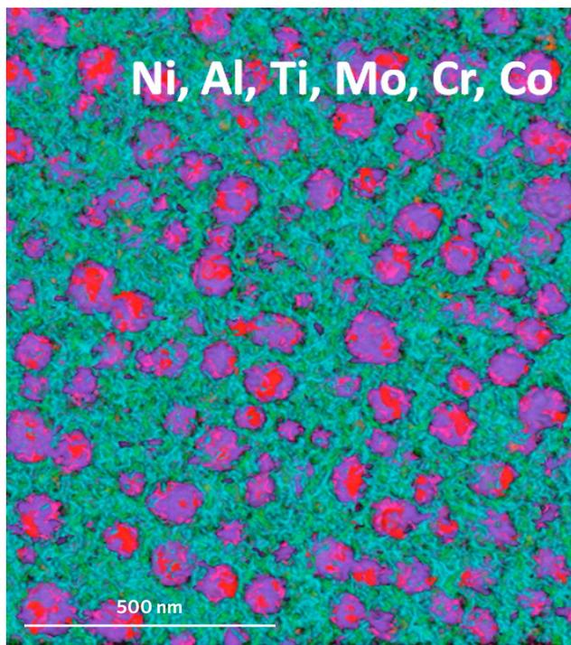
Figure 1a. Compositional map of the Ni based superalloy sample: 2D EDS multi-element compositional map of 512 × 512 pixels. Acquired in <5min.
