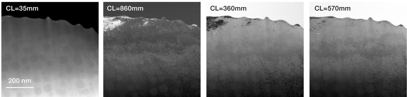
Figure 4. Series of S/TEM images with HAADF STEM detector at selected camera length (CL) values.
