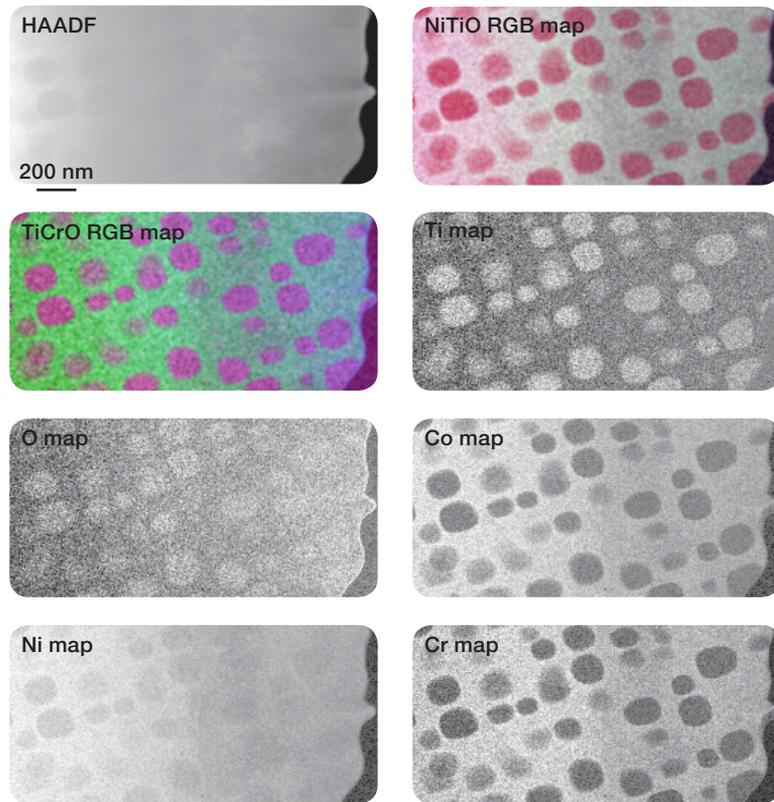
Figure 6. 2D EELS compositional maps acquired with Gatan EELS spectrometer. These maps of 280x235 px were acquired in 30 min. and post-processed separately.
