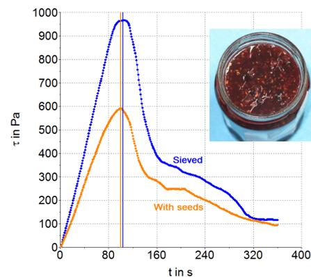
Figure 4: Comparison of FL 22 vane rotor yield stress measurements at 0.05 rpm for a sieved raspberry jam (blue curve) and raspberry jam with seeds (orange curve, inserted image).
