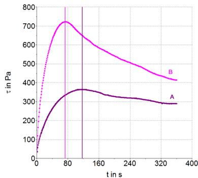
**Figure 5: FL 22 vane rotor yield stress measurements at 0.05 rpm for chocolate hazelnut spread products A and B.**
