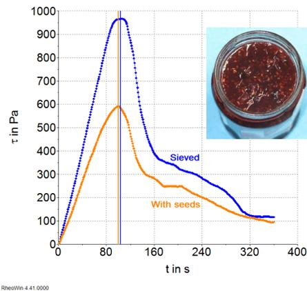
Figure 4: Comparison of FL 22 vane rotor yield stress measurements at 0.05 rpm for a sieved raspberry jam (blue curve) and raspberry jam with seeds (orange curve, inserted image).
