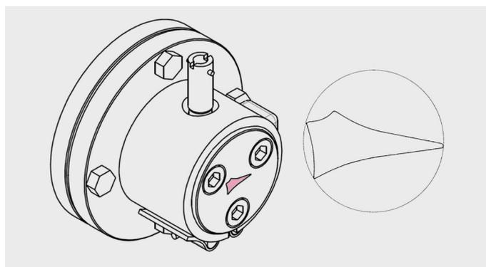
Figure 1: Schematic drawing of a Garvey die and its profile.
