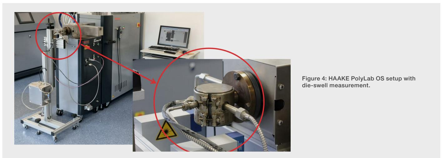
Figure 4: HAAKE PolyLab OS setup with die-swell measurement.
