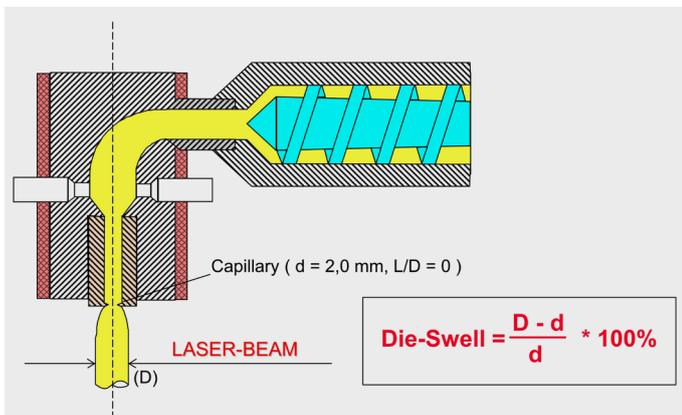
Figure 5: Schematic and calculation of die-swell measurement.
