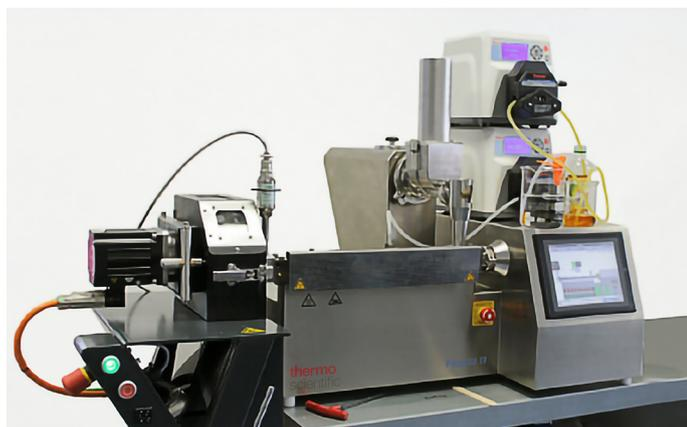
Figure 1: The Thermo Scientific Process 11 “Hygienic” Parallel Twin-Screw Extruder.
