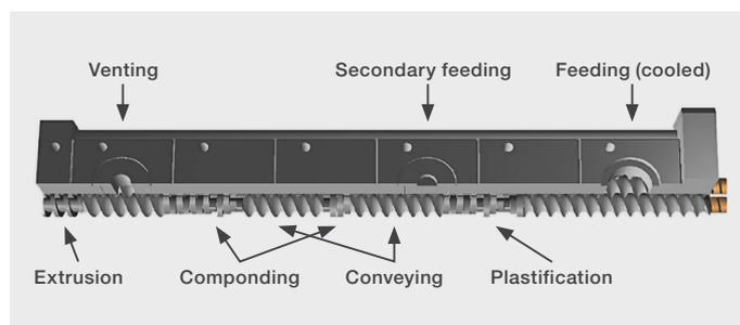
Figure 2: Schematic of a twin-screw extrusion.
