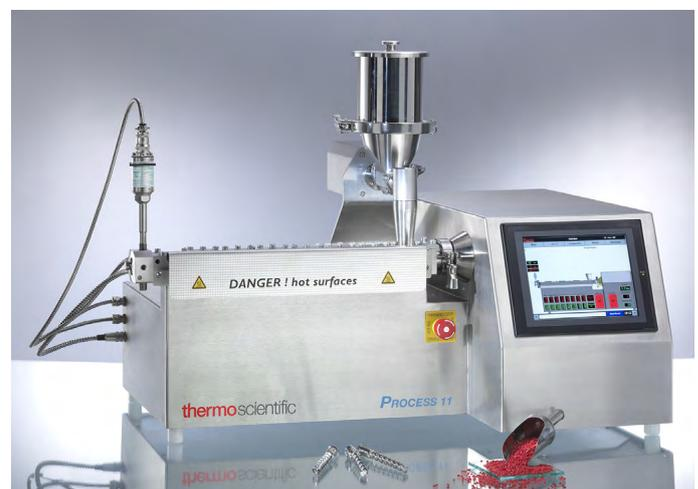
Figure 5: Thermo Scientific Process 11—11 mm lab scale screw compounder.
