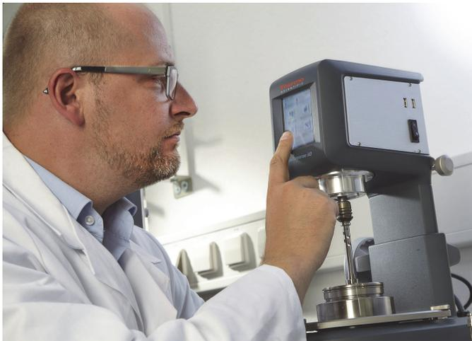
**Fig. 2:** HAAKE Viscotester iQ used as a standalone unit with internal measuring procedures, HAAKE Viscotester iQ RheoApp for extended measuring capabilities.
