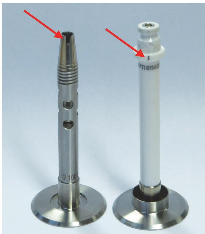
Fig. 1: Classical measuring geometry with a notched cone (left) and a Connect Assist measuring geometry with a mark on its ceramic shaft for defined mounting (right).
