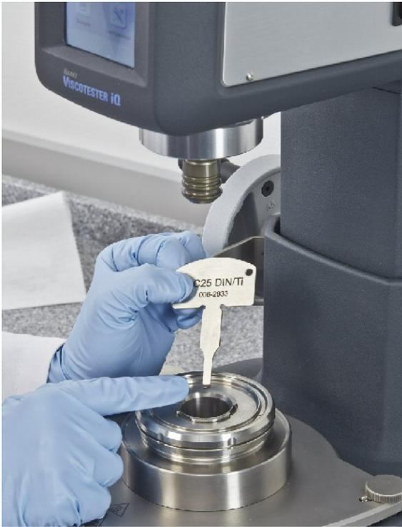
Fig. 4: Level gauge for coaxial cylinder geometries.
