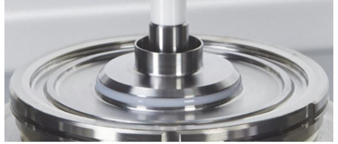
Fig. 7: Lower measuring plate TMP with a diameter chosen to match the upper geometry.
