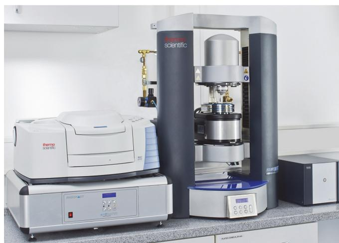
**Figure 1:** The HAAKE MARS Rheometer with Rheonaut module and Nicolet iS 10 FT-IR spectrometer.
