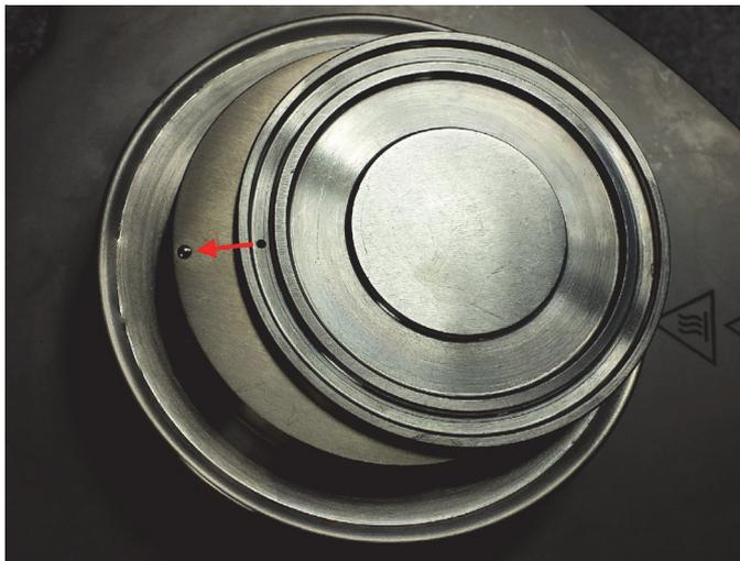
Fig. 2: For our PP- and CP-geometries, measuring plates TMP with the corresponding diameters are available. The notch under the mark on the TMP slides over the pin in the temperature control unit for easy and precise positioning.
