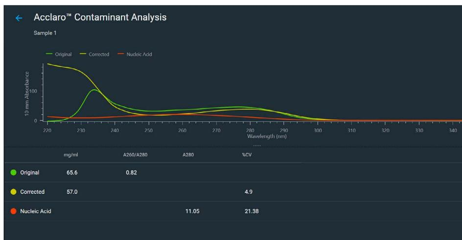
Figure 1: The Acclaro technology in the NanoDrop One/One<sup>c</sup> software identifies DNA contaminants in protein preparations in the Protein A280 application. The corrected spectrum is reported in yellow, the original spectrum is reported in green, and the contaminant spectrum is in orange.
