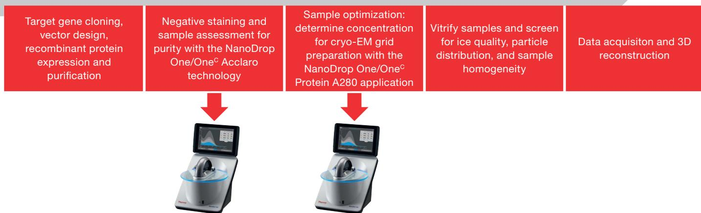
Figure 4: Cryo-EM workflow including the NanoDrop One/One<sup>c</sup> spectrophotometer integration for determining protein purity and concentration prior to application to the EM grid.
