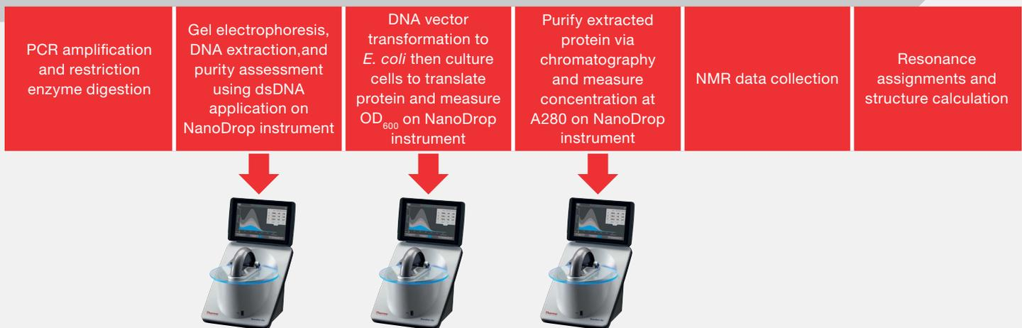
Figure 2: Workflow involving creation and purification of the DNA plasmid, measuring DNA concentration on the NanoDrop One/One<sup>c</sup> spectrophotometer, transformation of DNA vector to *E. coli* cells, culturing cells, measuring OD<sub>600</sub> on the NanoDrop instrument, and assessing purity and concentration after each purification method with the Protein A280 application and data is then collected via NMR.
