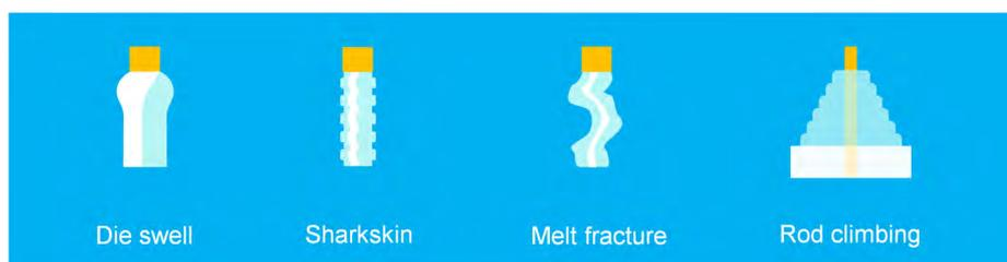
Figure 1: Typical flow anomalies of viscoelastic polymer fluids.
