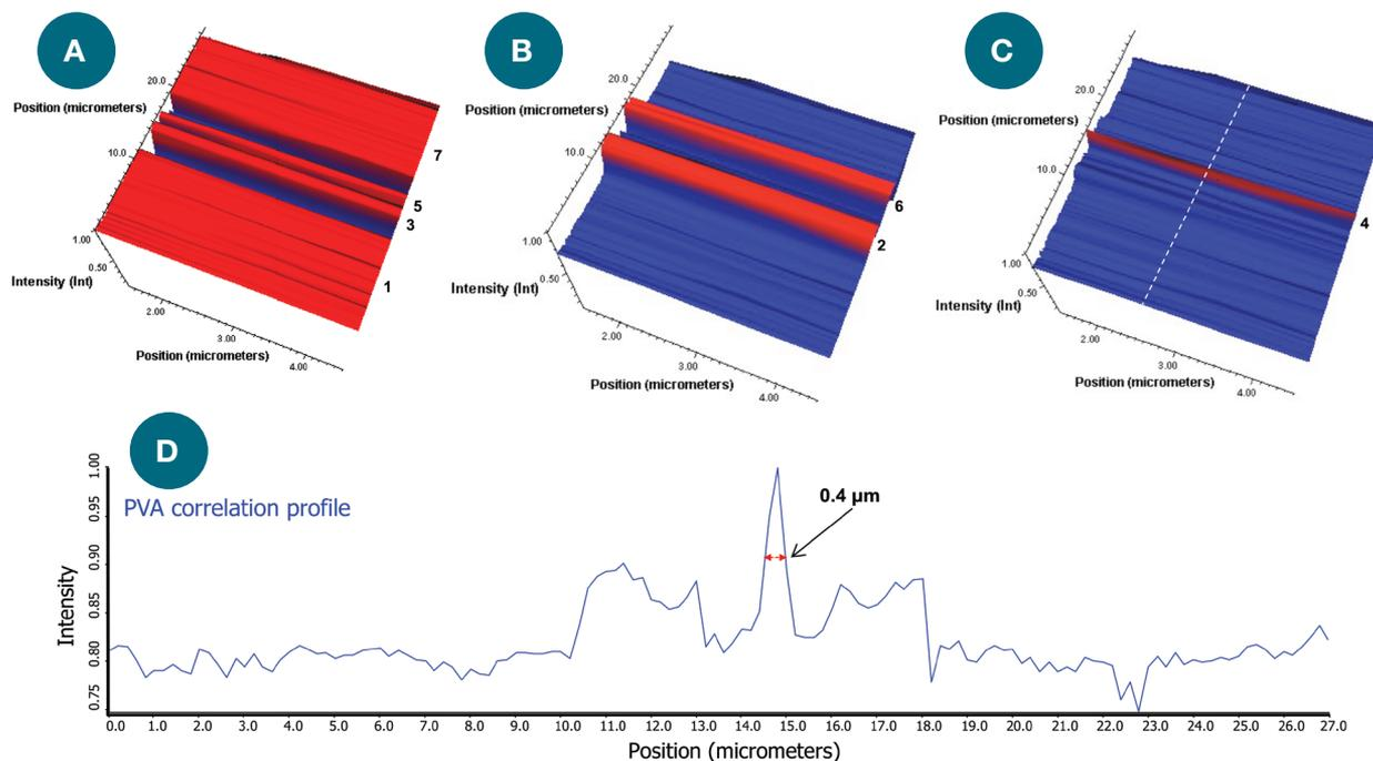
**Figure 2. 3-D Raman correlation images for microfilm B.** (A)-(C): Raman correlation images for PE, PP, and PVA, respectively. (D) Raman correlation profile obtained using a PVA reference spectrum on a line extracted from the area map (white dashed line on C).
