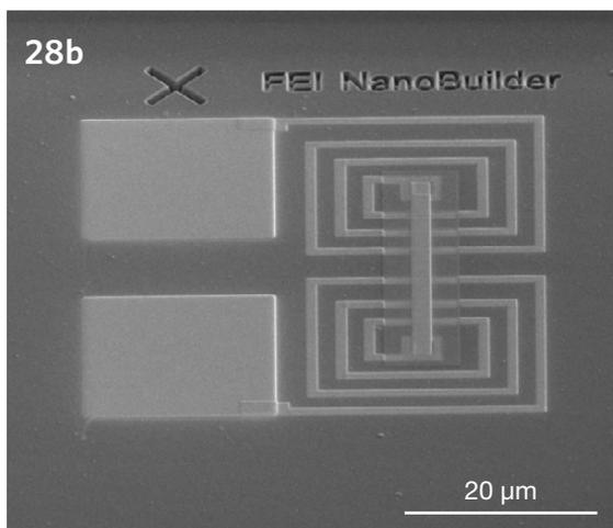
Figure 28. Same dual coil inductor device as the one presented in fig. 15. Its design (28a) consists of different layers, one for each of the building blocks of the device: deposition of a specific material, milling with a specific ion current, etc. Once the design is complete, NanoBuilder Software automatically executes the writing of all layers (28b).
