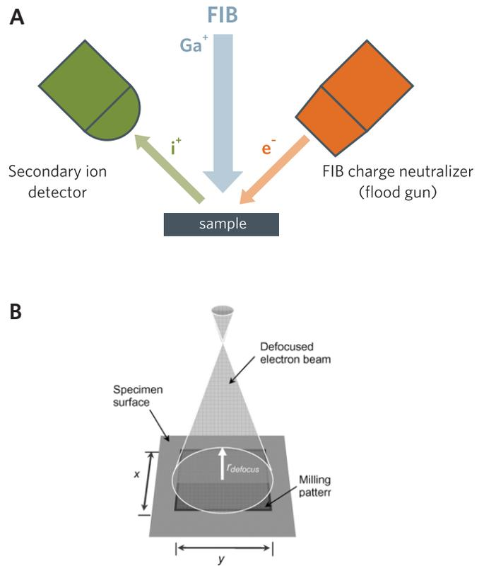
Figure 4. Solutions for efficiently neutralize positive charge build-up resulting from FIB milling on non conducting materials, such as a dedicated low energy electron flood gun (6a), or a defocused SEM beam irradiating the surface during FIB milling (6b) can be used in DualBeams.
