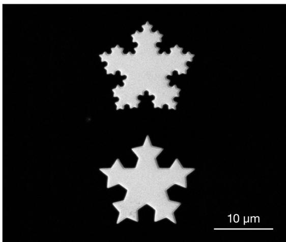
Figure 22. Electron beam lithography pattern in a resist, showing the precision build-up of a fractal pattern.
