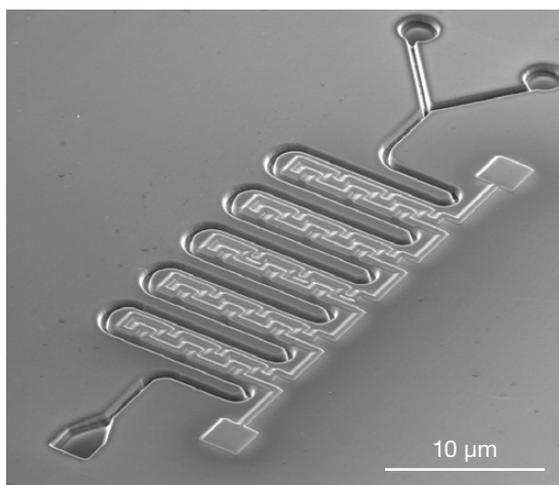
Figure 27. A photonic crystal pattern in InP, covering a total area of  $500 \times 100 \mu\text{m}^2$ , was split into 5 writing fields. The alignment crosses were FIB milled as part of the photonic crystal design and serve as a reference for the exact position of each field. The position of the crosses is registered after each stage move to align the pattern in the actual writing field accurately to the previous one.
