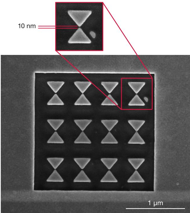
Figure 9. Nanoantennas in IR and VL - bowtie structures patterned on 40 nm Au/Si. Image courtesy of CIC Nanogune - Spain.
