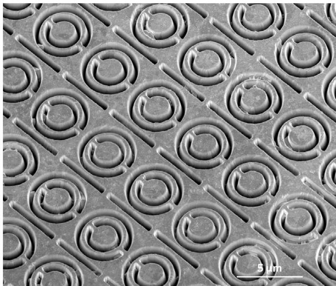
Figure 7a. A split-ring oscillator pattern directly milled using FIB. The FIB used a “vector scan” that allows the ion beam to be moved in the optimum direction for each portion of the pattern and allows multiple passes of the pattern to avoid any redeposition artifacts.
