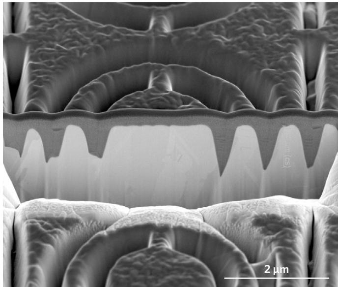
Figure 7b. A FIB-cut cross section through the split-ring oscillator.
