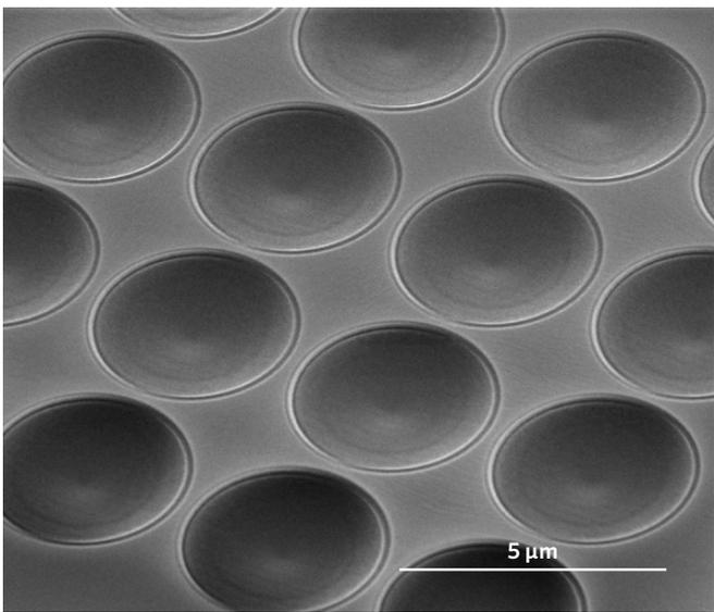
Figure 8. Secondary electron image of a micro-lens array milled into a silicon substrate. The lens shapes are accurately formed using our integrated patterning engine designed for advanced patterning.
