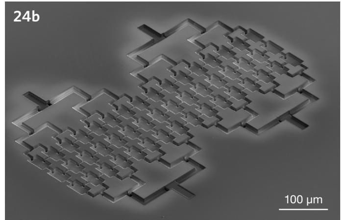
Figure 24. One millimeter long microfluidic device viewed from the NanoBuilder Software interface (a) and at an angle with the SEM, after completion of the automated FIB writing (b). As the FIB cannot write such a large device with high accuracy, NanoBuilder Software subdivides the design into smaller fields and precisely repositions and writes each of them. Here about 100 writing fields were used.
