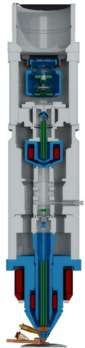
Figure 17. The Thermo Scientific™ Verios SEM and the Helios NanoLab DualBeam, formerly produced by FEI, feature unique integrated technologies that allow state-of-the-art electron beam lithography: a stable platform, highly precise and reproducible movements thanks to Piezo stages (a), and a high-resolution FEG column with conjugated fast beam blower (b).
