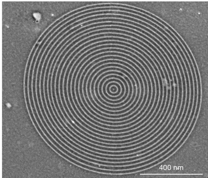
Figure 12. Electron beam induced direct deposition of Pt lines, arranged in concentric circles. Each line has a width of 7 nm, the pitch between two lines is 22 nm.
