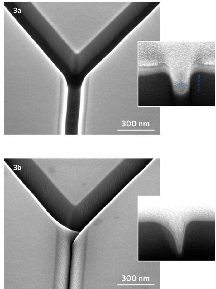
Figure 3. Detail of a nanofluidic trench (the insert shows a FIB cross section of the trench imaged in a TEM). Optimized FIB patterning strategies (3a) yield good profile control and clean, vertical sidewalls. Typical e-beam lithography patterning strategies (3b) do not account for the specificities of the ion beam milling process, therefore yielding redeposition and/or unwanted milling.
