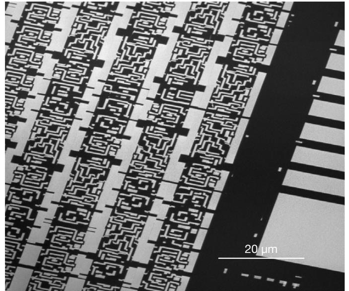
Figure 19. Example of electron beam lithography of an electronics device, accurately written at high speed with a high current (1 MHz writing speed with 1.4 nA beam current).
