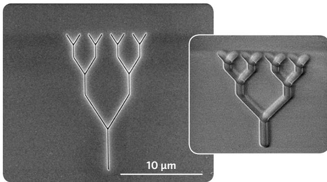
Figure 5. A flood of low energy electrons is used to neutralize the charge built up on the surface by scanning with the positively charged gallium ion. A nano-fluidic channel can be cut perfectly even in a quartz substrate. Without charge neutralization (see image insert) the ion beam is deflected during milling and results in an inaccurate cut.
