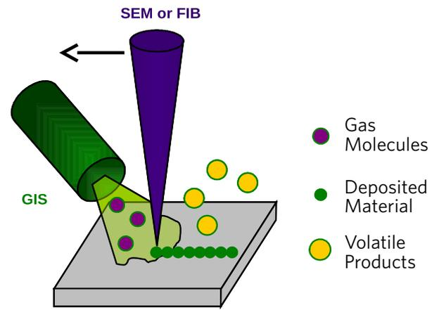
Figure 11. Illustration of FIB/SEM beam chemistry used to deposit material onto the surface of a sample.
