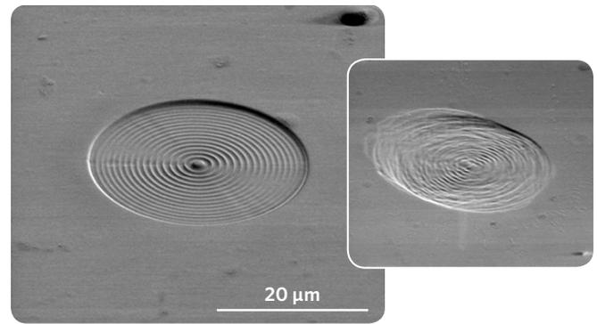
Figure 6. Using charge neutralization a circular pattern can be perfectly milled in glass. When the charge neutralization is turned off (see image insert) the ion beam moves erratically during milling and results in poor milling.
