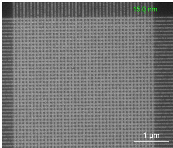
Figure 21. Series of crossing horizontal and vertical lines, transferred in an electron beam lithographic resist using a Helios NanoLab DualBeam. The line width is 15 nm.
