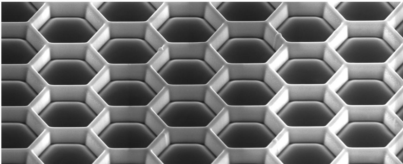
Figure 1. Secondary electron image of a honeycomb structure milled into a silicon substrate using the FIB on a Thermo Scientific™ DualBeam instrument. The hexagonal shapes are accurately formed using the Thermo Scientific integrated patterning engine designed for advanced patterning.
