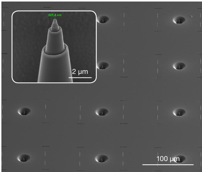
Figure 25. Automated preparation of an array of 10 x 3 AFM tips, with a pitch of 150 μm, using NanoBuilder Software. For each tip, FIB currents from 20 nA down to 10 pA were used, including a beam re-alignment after each current change using the fiducials. The inset shows the detail of one tip.
