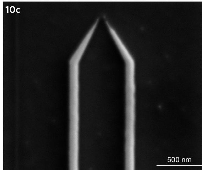
Figure 10. 10x10 array of IF plasmonic waveguides, min. feature size < 50 nm, written on a 40 nm Au/Si sample. (a) full array (b) one waveguide (c) waveguide detail. Images courtesy of CIC Nanogune - Spain.
