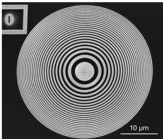
Figure 23. A zone plate diffraction grating written and imaged with electron beam lithography using low vacuum conditions to eliminate any charging artifacts in the patterning or the imaging.
