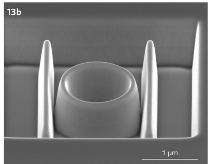
Figure 13. A ring oscillator milled by FIB into GaAs, without (13a) and with (13b) an enhanced etch beam chemistry. This specific beam chemistry passivates the milled surface and prevents the formation of gallium droplets.
