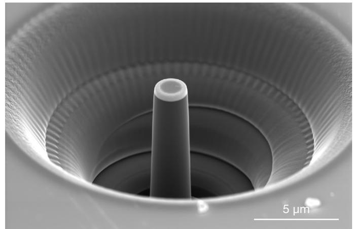
Figure 26. Non-tapered pillar for micro-mechanical testing. An automated multi-step FIB milling process, driven by NanoBuilder Software and consisting of a sequence of decreasing beam currents and alignments, was used for optimum shape control.
