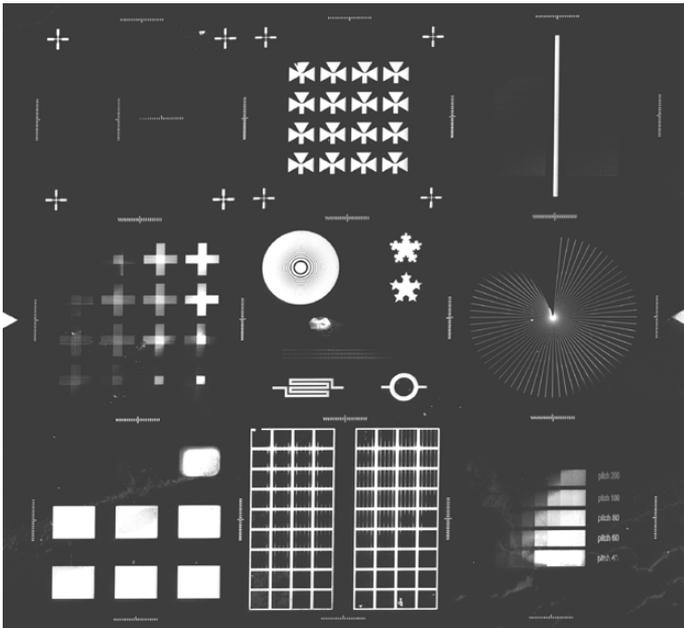
Figure 18. An electron beam lithography test pattern made over a 300  $\mu\text{m}$  x 300  $\mu\text{m}$  area. The high accuracy of the Piezo stage is used to place patterns in a serpentine fashion, starting horizontally at the bottom left. An array of 3 x 3 fields (100 x 100  $\mu\text{m}$  each) were stitched with an accuracy of >300 nm. The Vernier scales indicate stitching positions (displacement of 20 nm per tick in opposing scales. Tick width 200 nm).
