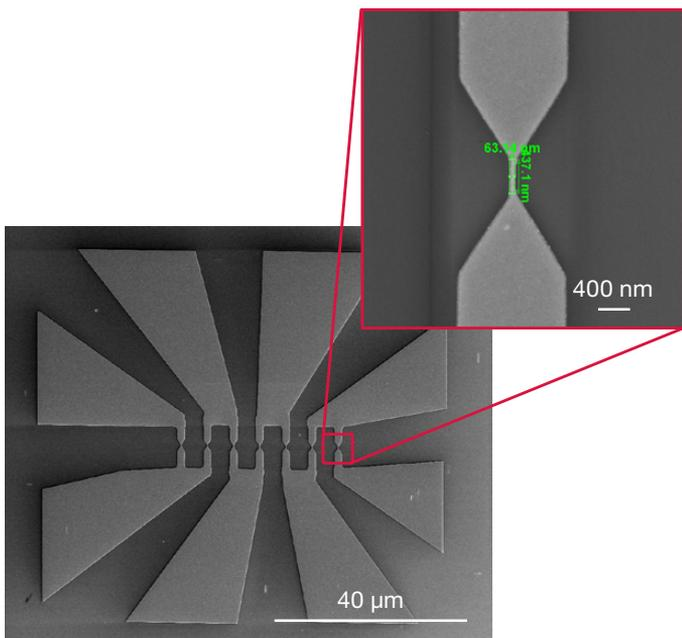
Figure 20. Electromigration structure created by electron beam lithography. NanoBuilder Software was used to drive the electron beam to transfer the structures on the resist.
