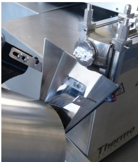
*Figure 6 - Eyecon<sub>2</sub> Particle Analyser with Integration Device in-place on Pharma 11 Extruder in Granulation Mode (View 1)*
