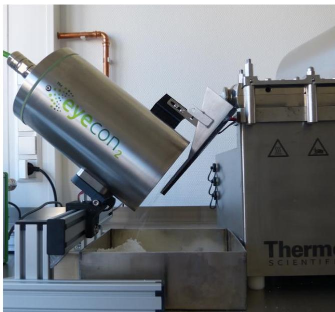
*Figure 7 - Eyecon<sub>2</sub> Particle Analyser with Integration Device in-place on Pharma 11 Extruder in Granulation Mode (View 2)*
