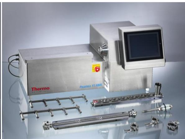
Figure 3 - Pharma 11 Extruder Disassembled for Cleaning
