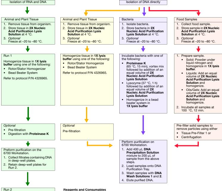
Isolate DNA from tissue filtrates using TransPrep chemistry and reagents.
