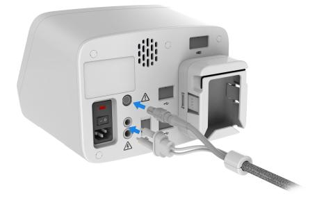
Be sure to align the ridge on the connector of the cable with the groove on the port of the Neon<sup>™</sup> NxT device.
