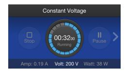
7. The run screen displays the run parameters in real time during the run. The center dial displays a countdown timer for the method.
