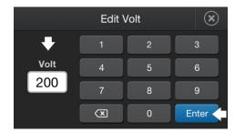
**4.** Set the operating mode parameter (Constant voltage) by entering the value in the Volt field, then select Enter.
