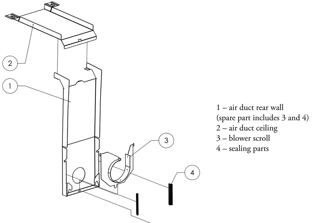
**Figure 4-4. STERI-CYCLE i160 LK Air Duct Assembly Components**
