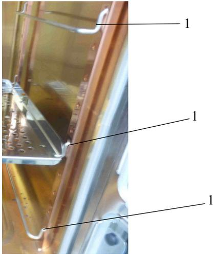
Insert the shelf supports (1) in the lower, center and upper **rectangular** holes of the support rails.
