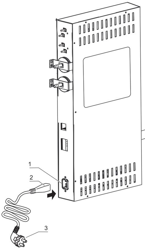
**Figure 4-15.** Power Supply Connection
