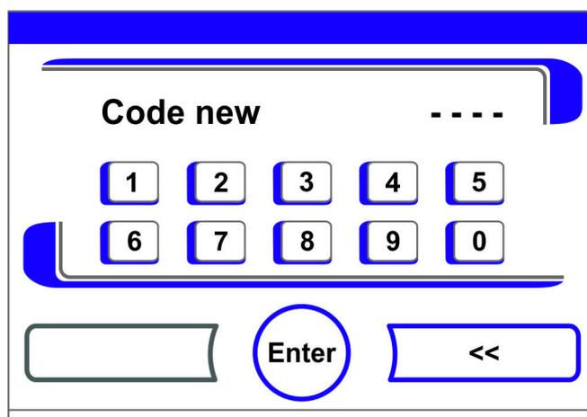
**Figure 6-20.** Changing the Keypad Lock Code
