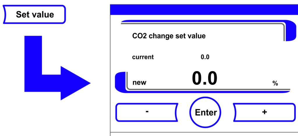
**Figure 6-10.** Setting the CO<sub>2</sub> Set Value
