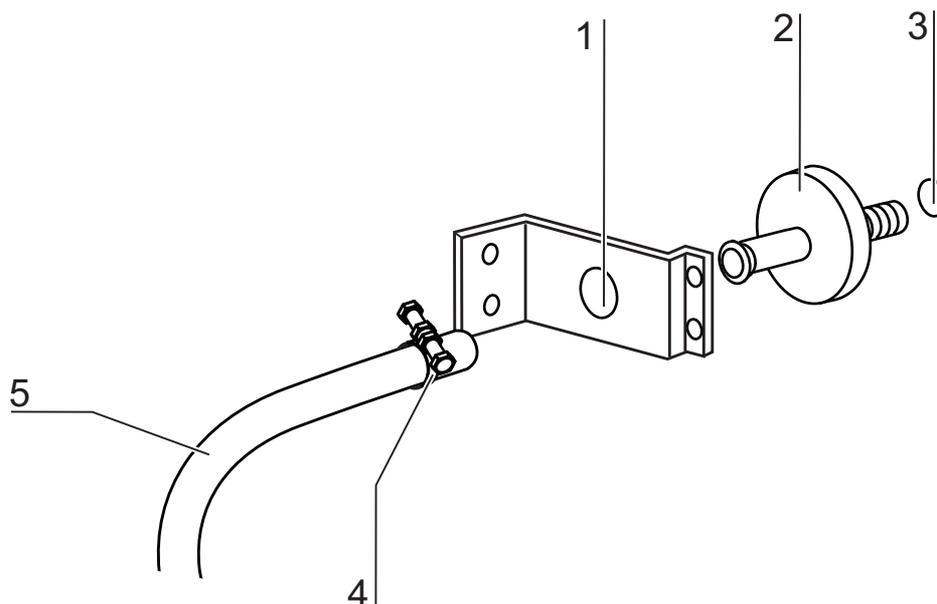
**Figure 9-8.** Gas Inlet Filter Installation
