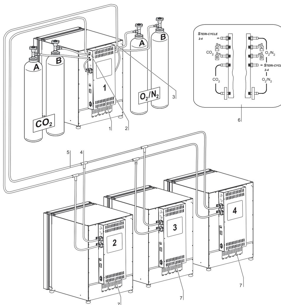
**Figure 3-3.** Looped-through Gas Supply *STERI-CYCLE i160 LK / STERI-CYCLE i250 LK*
