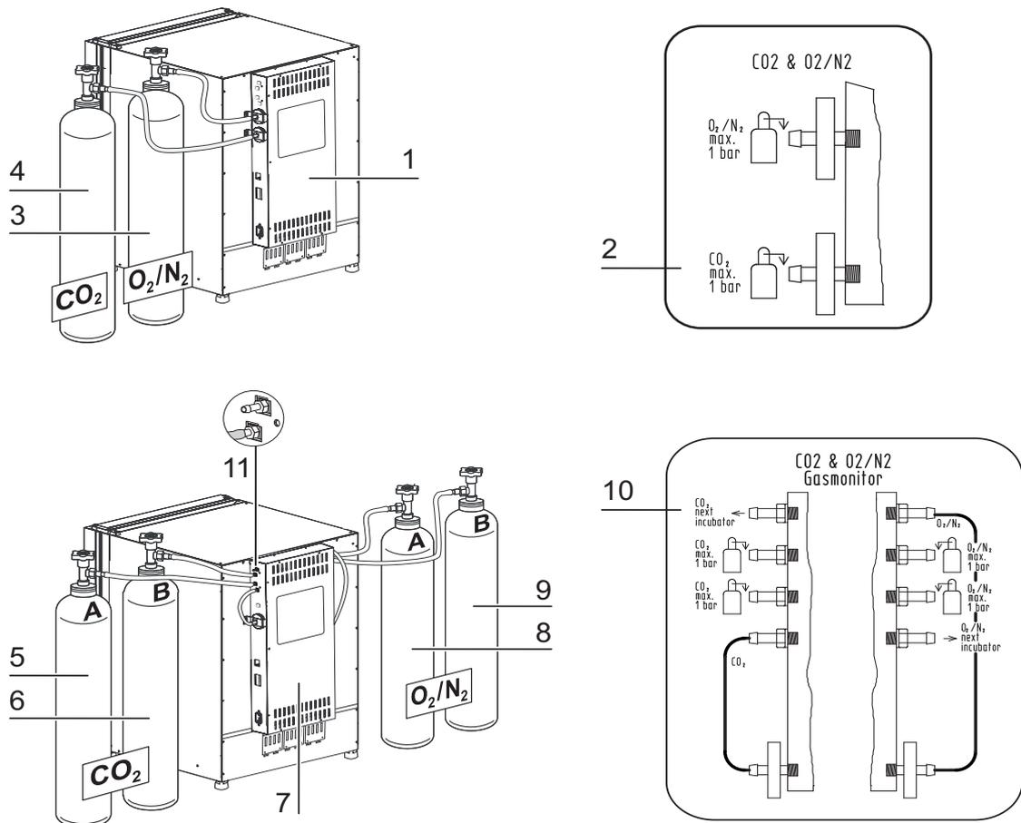
**Figure 3-2. STERI-CYCLE i160 LK / i250 LK Rear View**
