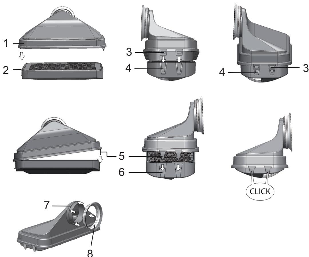
**Figure 4-5.** Assembling the HEPA-Filter and the Airbox
