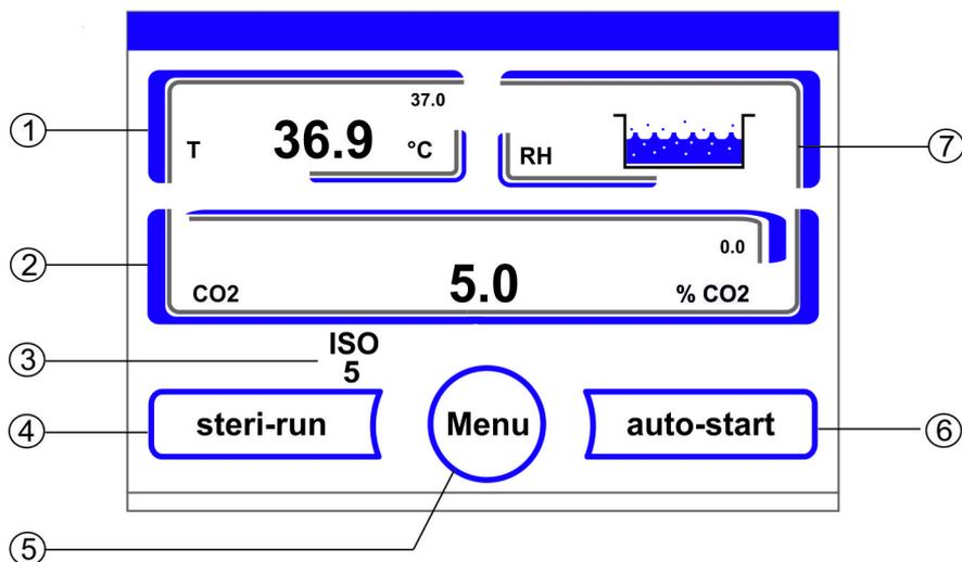
**Figure 6-3.** iCan™ Touchscreen without O<sub>2</sub>/N<sub>2</sub> Gas Supply
