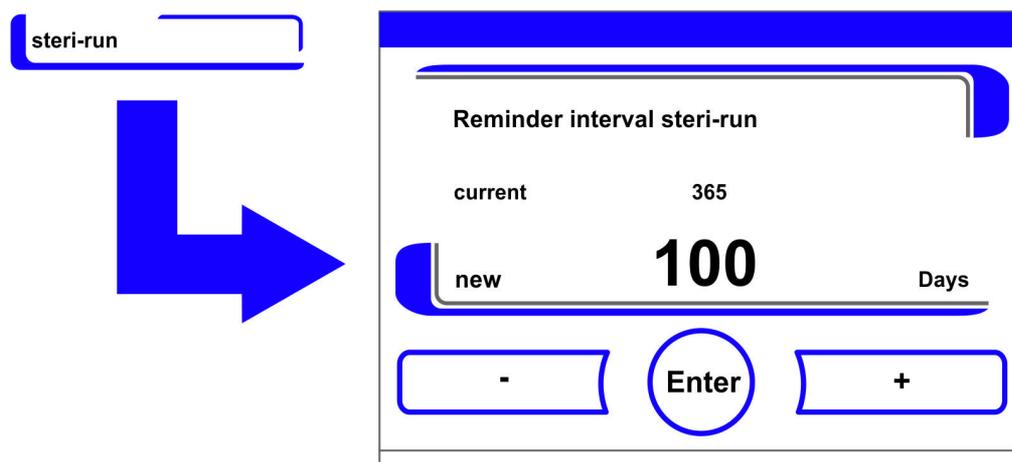
**Figure 6-30.** Setting the Reminder Interval for Steri-Run
