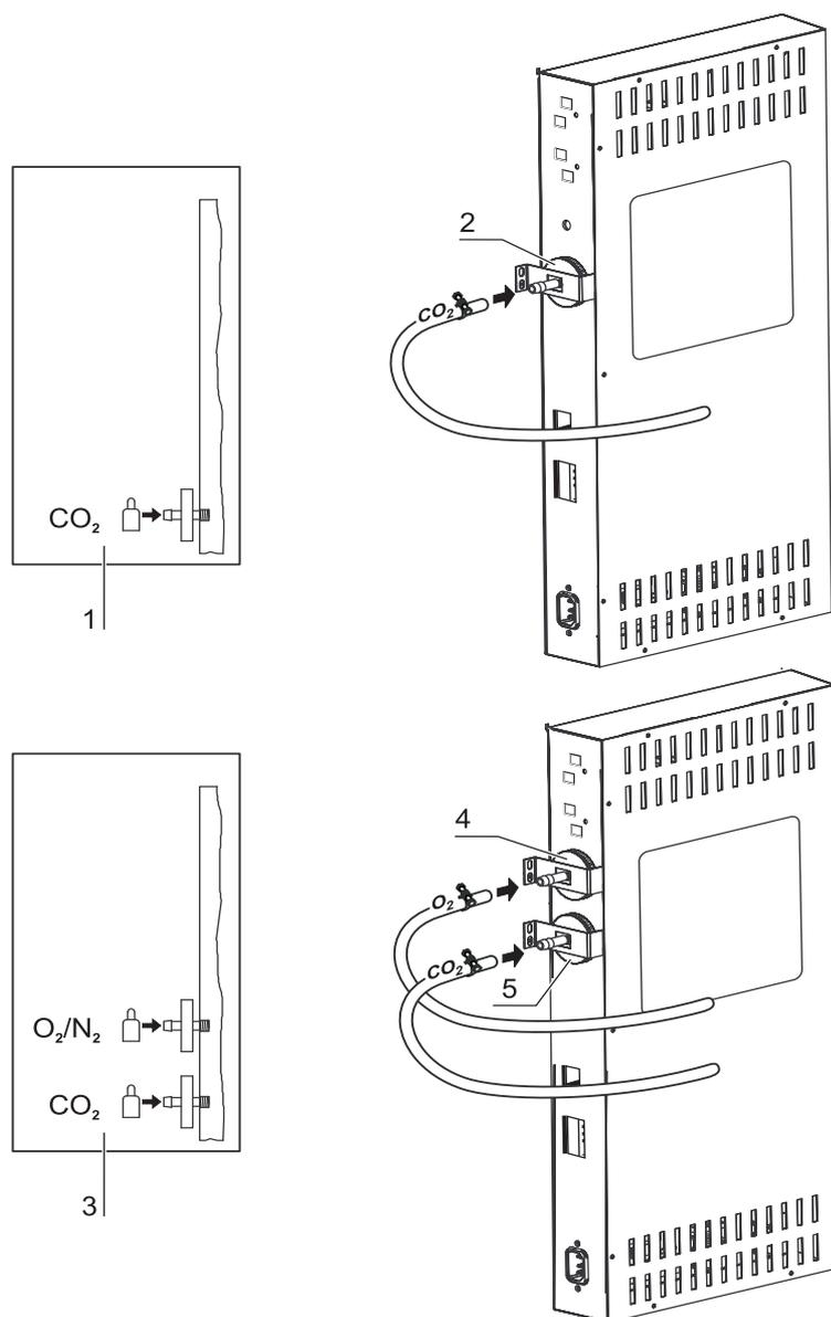
**Figure 4-12.** Gas Connection without Gas Monitoring System
