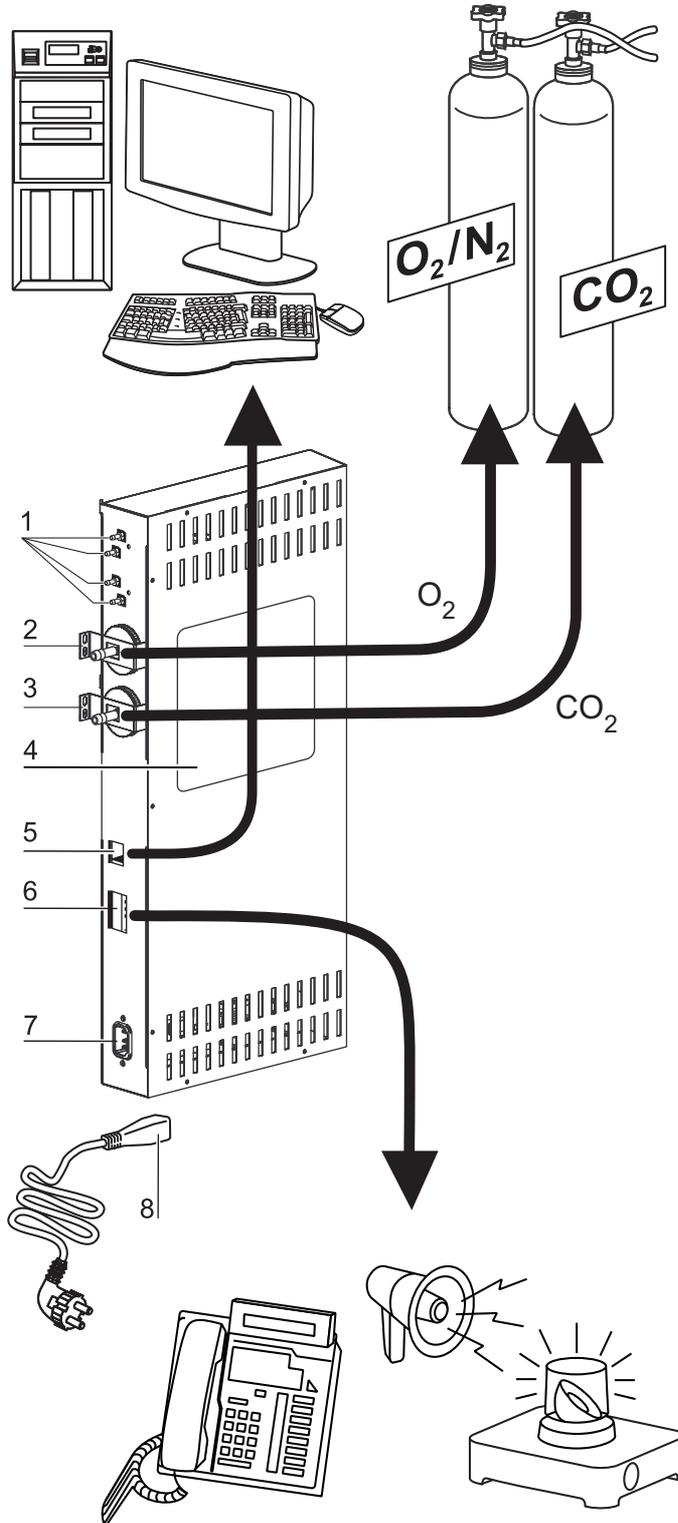
Figure 3-9. Interfaces (Right Side of Control Box)
