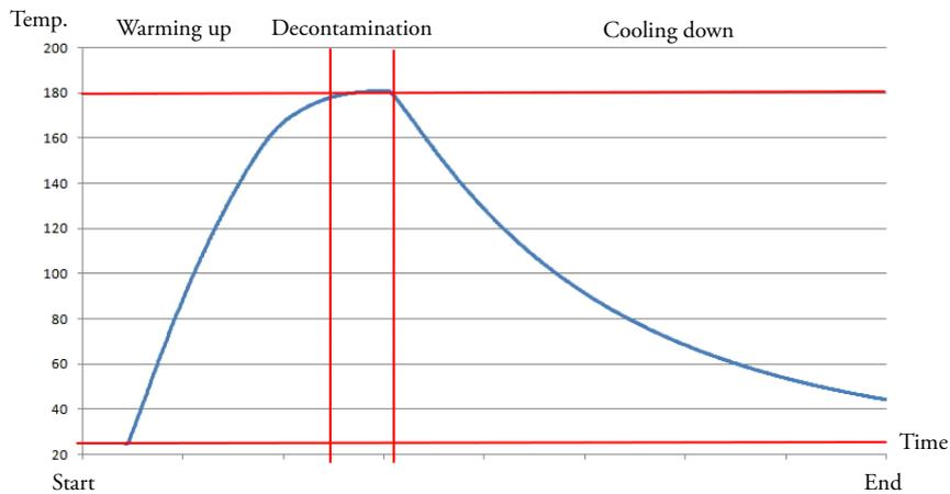
Figure 8-4. Decontamination Routine Phases
