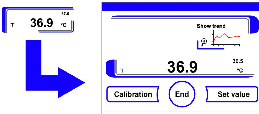
**Figure 6-7.** Temperature Display Field and Temperature Selection Menu
