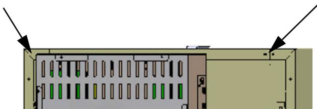
**Figure 2-6.** Removing the Screws for the Wall Brackets
