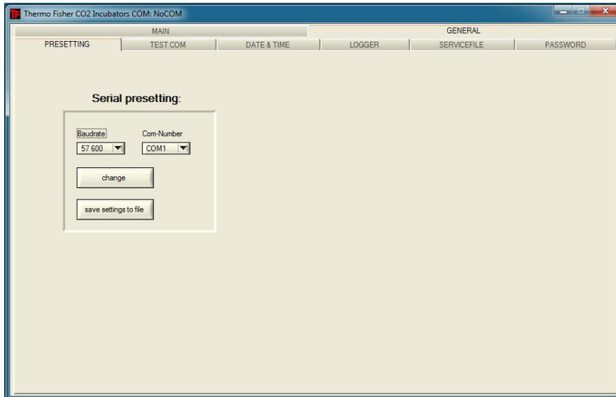
1. Select a transmission speed within the range of 9,600 to 115,200 baud.
