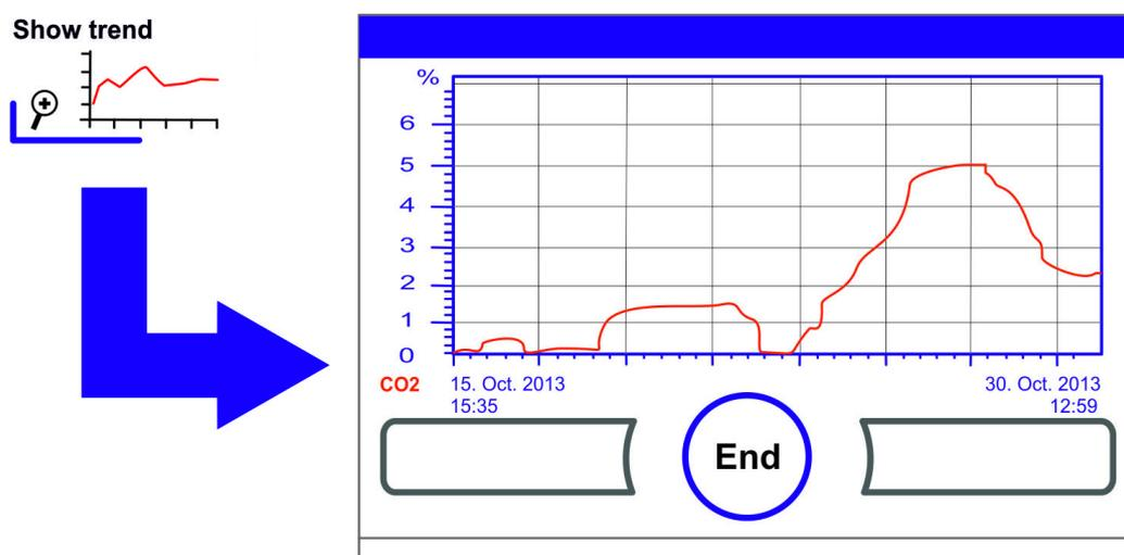
**Figure 6-50.** Invoking the CO<sub>2</sub> Concentration Graph Display
