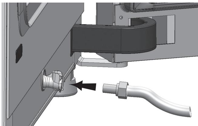
**Figure 8-1.** Fill and Drain Valve of Water Reservoir
