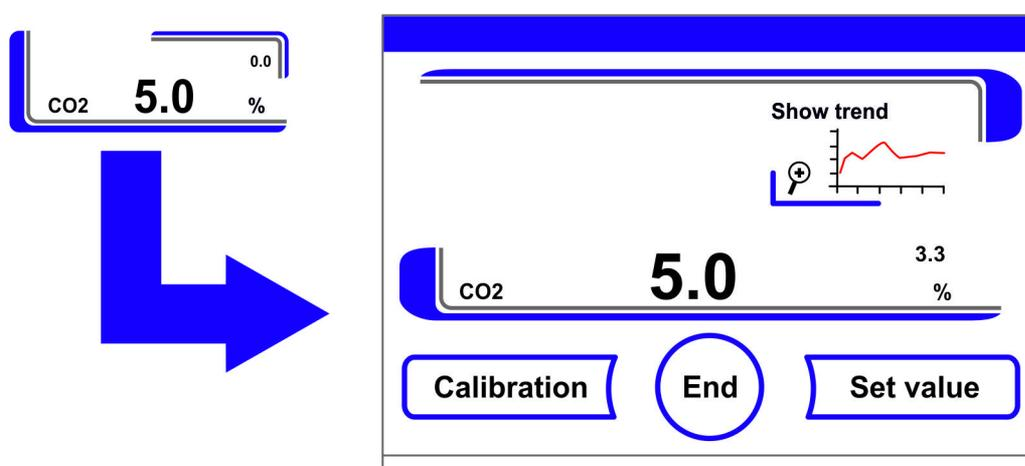
**Figure 6-9.** CO<sub>2</sub> Display and CO<sub>2</sub> Menu
