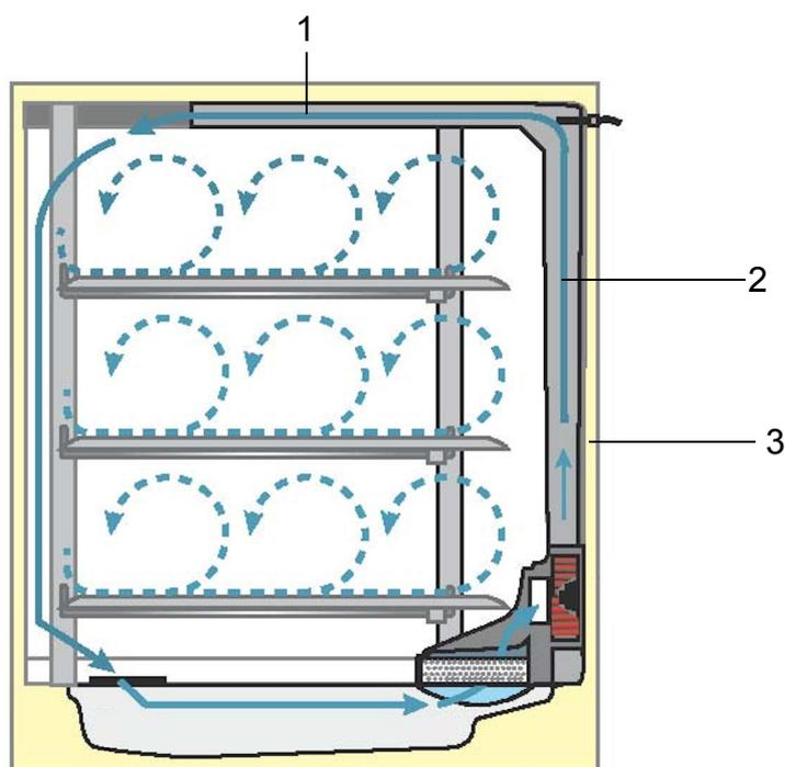
**Figure 3-5. Air Duct**
