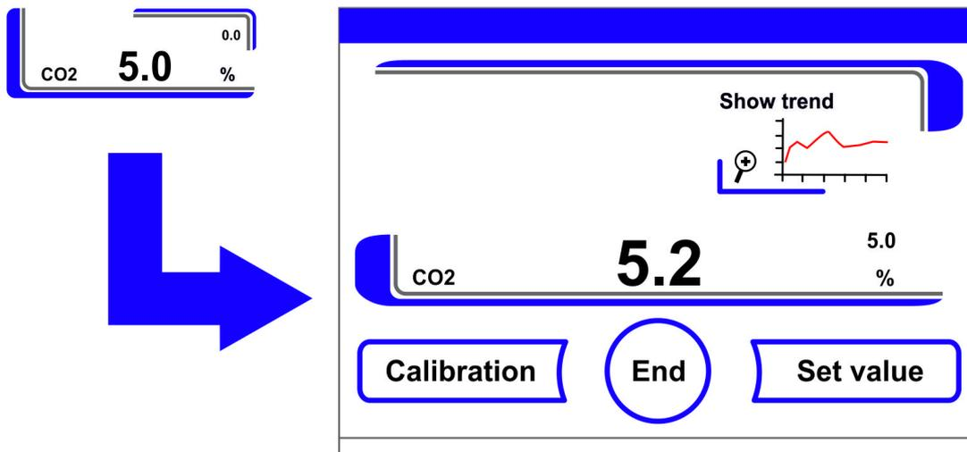
**Figure 6-49.** Invoking the CO<sub>2</sub> Concentration Graph Display
