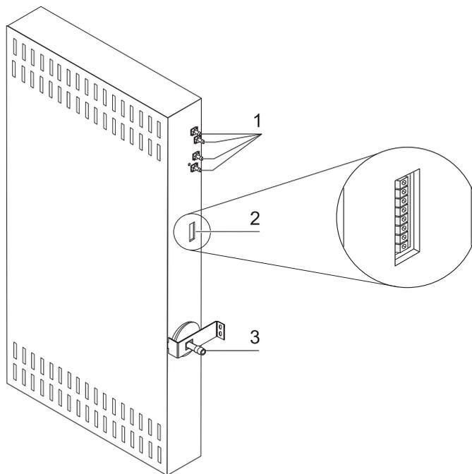
**Figure 3-10.** Optional Interfaces (Left Side of Control Box)
