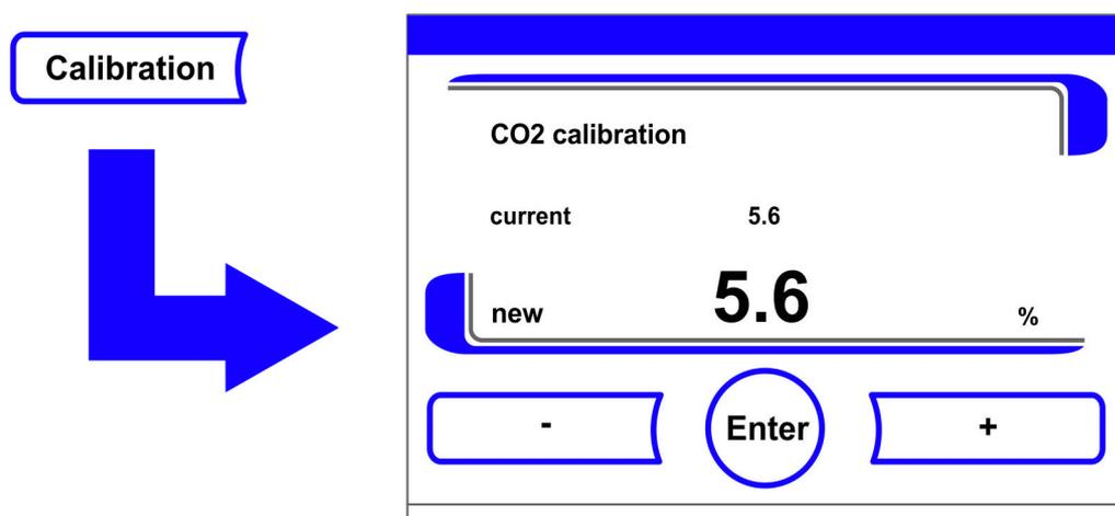
**Figure 9-5.** CO<sub>2</sub> Calibration Procedure
