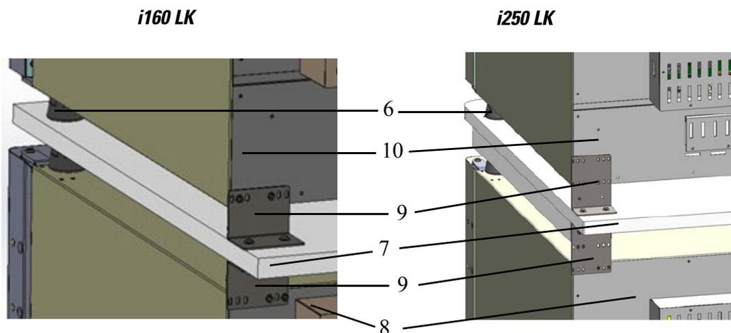
**Figure 2-5.** Fastening the Adapter Plate to the Lower Unit
