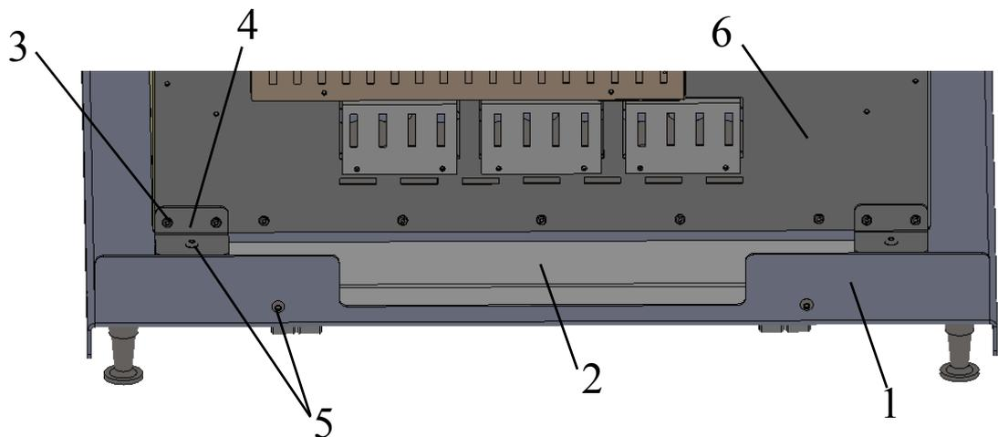
**Figure 2-10.** Fixing device on support stand with counter weight
