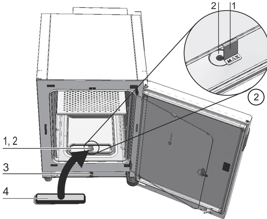
**Figure 4-2.** “MAX” Fill Level Indicator and Pre-Filter
