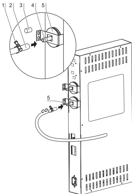
**Figure 4-11.** Installing Gas Pressure Hoses
