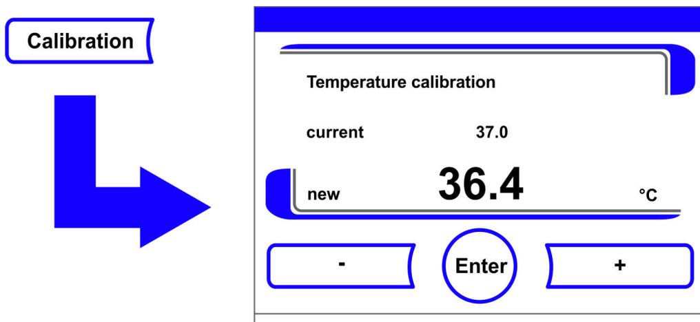
**Figure 9-3.** Temperature Calibration Procedure
