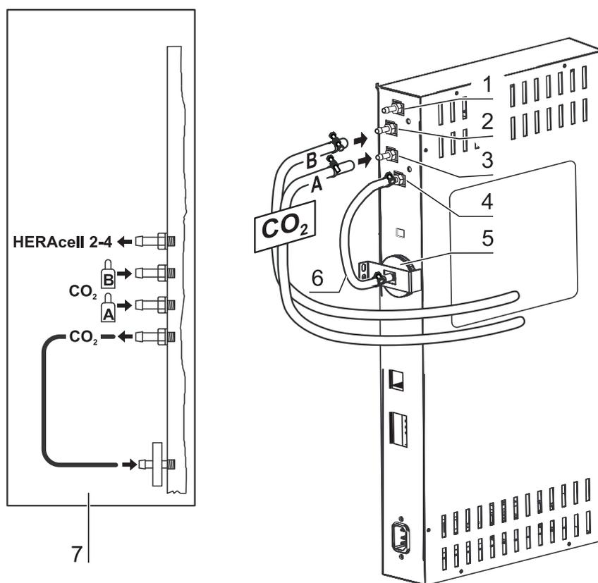
**Figure 4-13.** CO<sub>2</sub> Connection with Gas Monitoring System (Optional)
