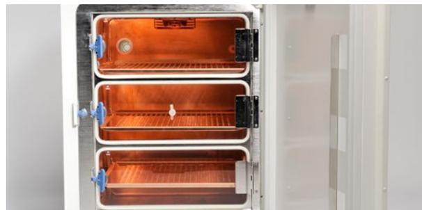
**Figure 3.** The segmented inner doors are standard on every Thermo Scientific Heracell tri-gas incubator, allowing access to individual areas and further reducing potential for incubator contamination. The zirconium oxide sensor provides fast recovery to desired hypoxic conditions.
