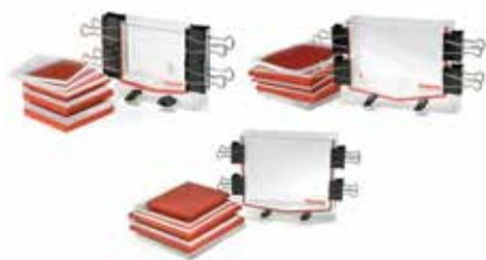
**Includes:** Casting stand with base port, spacer placer, foam, acrylic spacer plates, four binder clamps, front plate, 2 wing knobs and blocking plate
