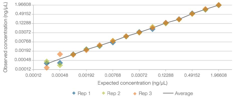
**Figure 5. Observed sample replicate concentrations for the sensitivity dilution series.** The y-axis is on a log<sub>2</sub> scale.
