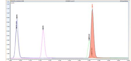
Figure 6. Chromatogram of both transitions of 3 MCPD and the calibration curve from 10 to 500 250 µg/kg
