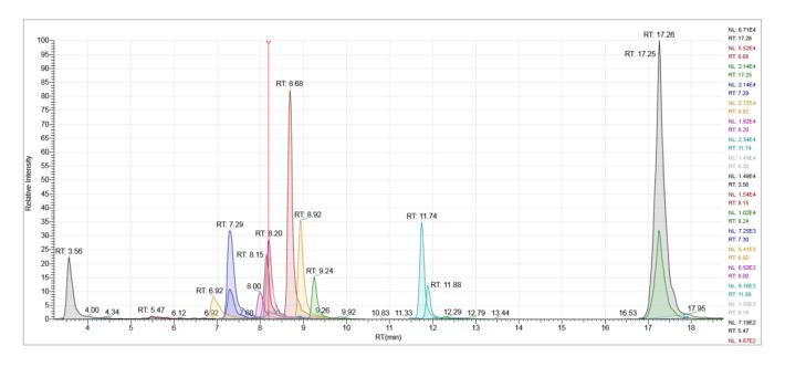
Figure 2. SRM chromatograms of 16 polar pesticides (10 µg/L each).
