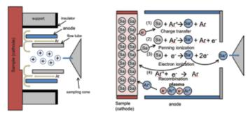
Figure 1. Schematics of a fast flow GD-MS source (courtesy of Dr. Sehoon Jung, Research Institute of Industrial Science and Technology (RIST), Pohang, South Korea).
