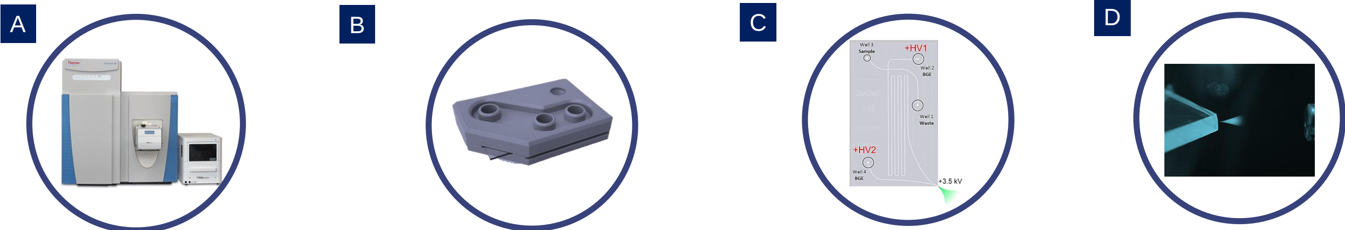
FIGURE 1: (A) ZipChip source interface that mounts onto mass spectrometer, and autosampler for automatic injections. (B) Picture of ZipChip device. (C) Picture of chip microfluidic architecture integrating capillary electrophoresis and electrospray mass spectrometry. (D) Picture of electrospray plume illuminated with green laser.
