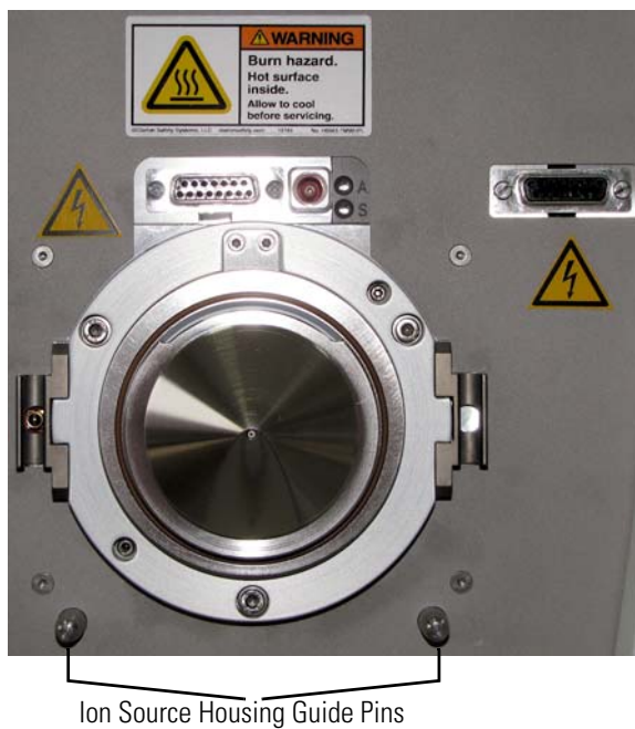
Figure 8-8. Ion source mount showing ion source housing guide pins
