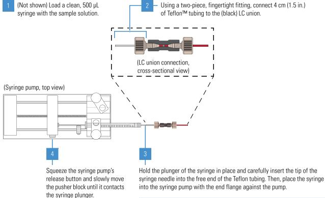
**Note** If necessary, use the syringe needle tip to enlarge the opening slightly in the end of the Teflon tubing.
