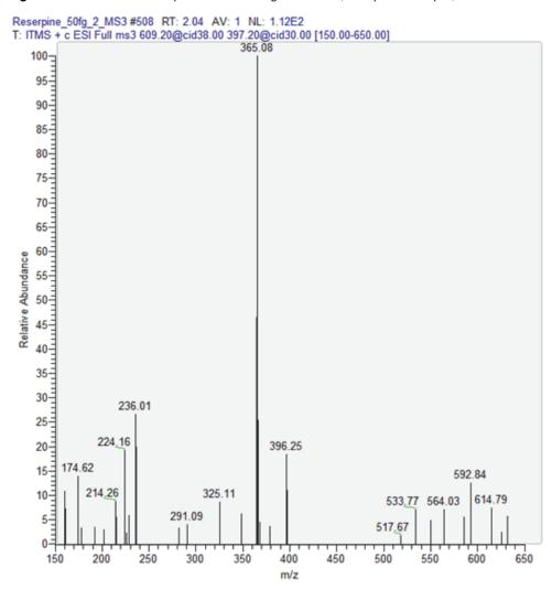
**Figure 20.** CID-MS<sup>3</sup> scan spectrum with fragmentation (reserpine example)
