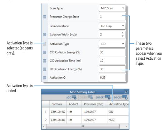
Figure 26. Activation Type selected and added to the MS<sup>n</sup> Setting Table (CID example)
