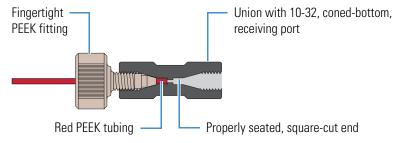
Figure 2. Proper connection for the PEEK tubing and fitting (syringe adapter assembly)
