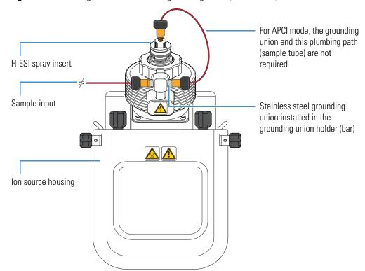
Figure 4. Plumbing connections for the grounding union (H-ESI mode)
