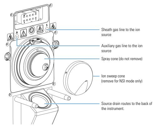
Figure 1. MS ion source mount assembly and ion sweep cone
