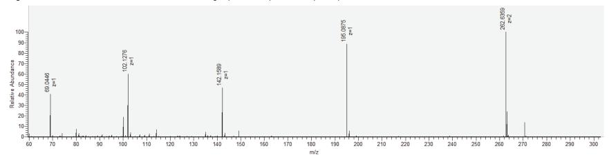
Figure 11. FlexMix calibration solution's low-mass range spectrum in positive ion polarity mode
