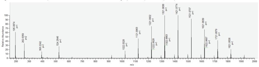
**Figure 9.** Traditional n-Butylamine calibration solution's normal mass-range spectrum in positive ion polarity mode
