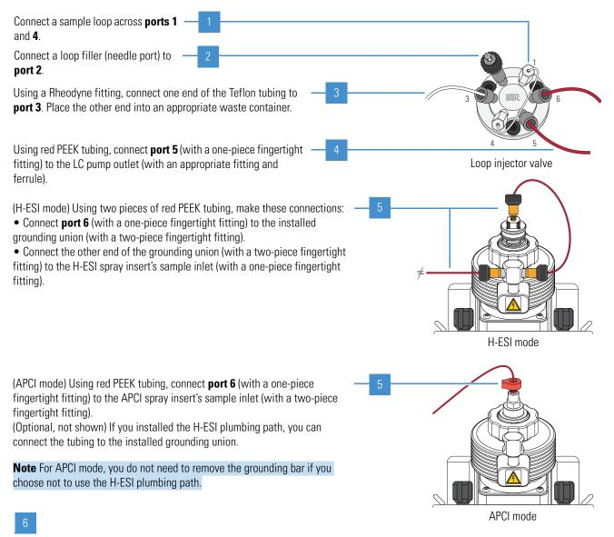
(Not shown) Load a clean syringe with the sample solution, carefully insert it into the needle port that is installed in **port 2**, and then slowly press the syringe plunger.
