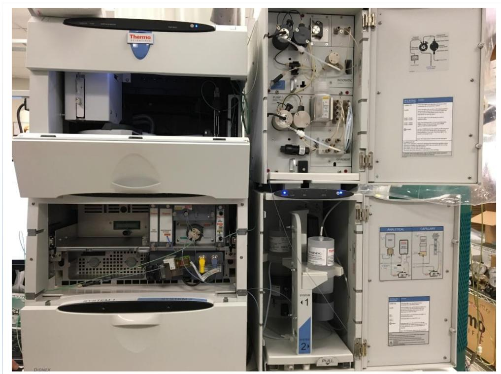
1. Fill a 2 L eluent reservoir bottle with ASTM filtered, Type I (18-megohm) degassed deionized water. Connect the reservoir to the eluent inlet line of the pump. Keep the water blanketed under an inert gas (helium or nitrogen).
