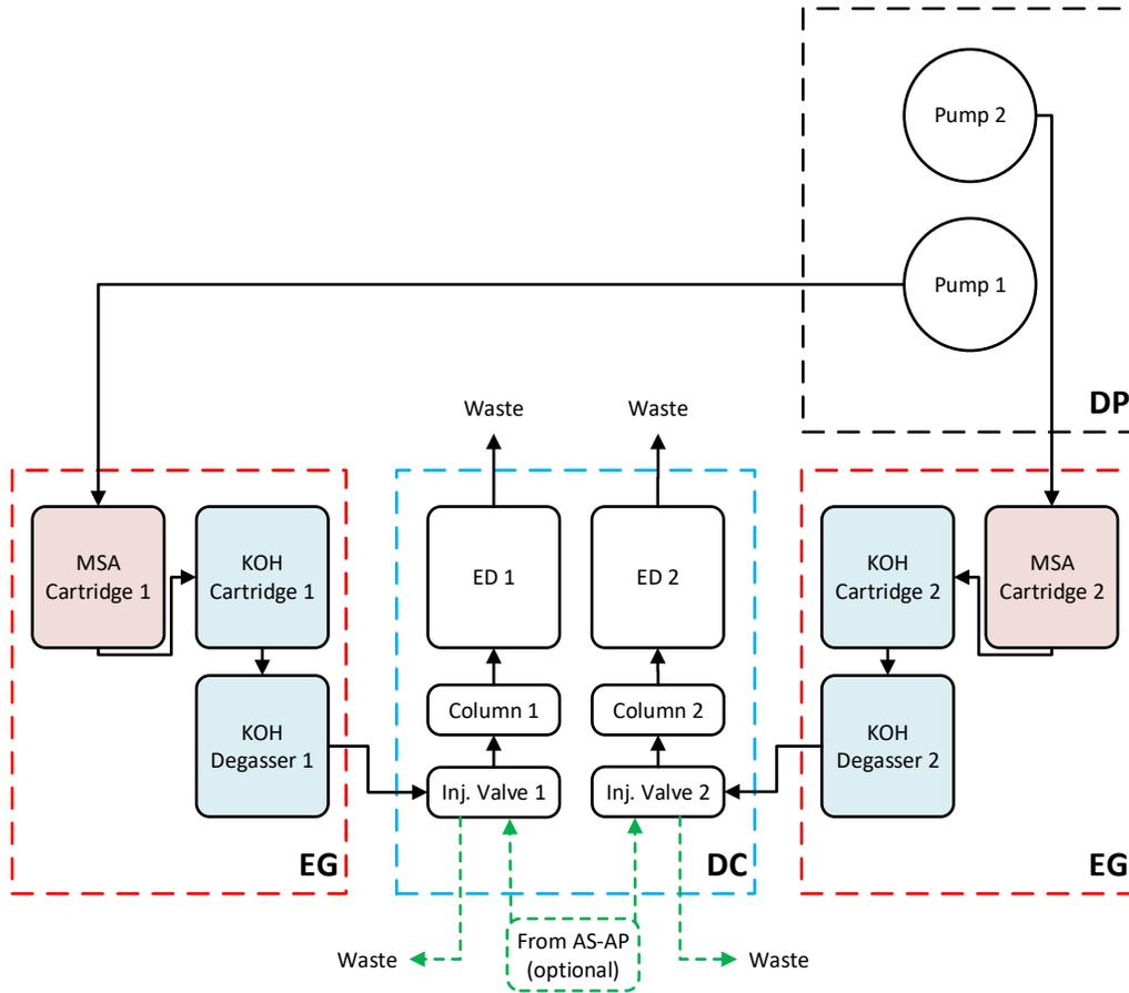
**Figure 12 Vacuum Tubing Connection on the Liquid Trap for ICS-6000 System Dual EGC Mode with 1-mm/1-mm Dual Channels**
