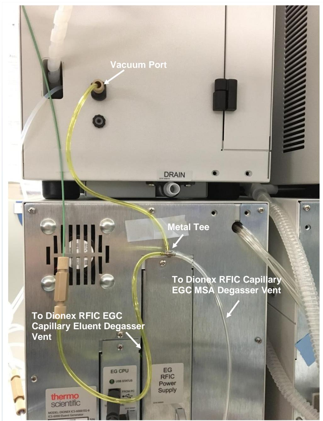
Figure 8 Vacuum Line Connections for Dual EGC Mode, 0.4-mm Column
