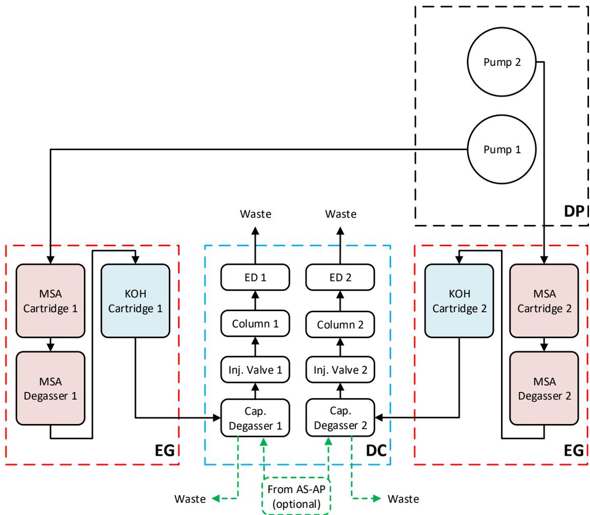
Figure 21 Dual Channel Dual EGC Mode Vacuum Connection, 0.4-mm Column
