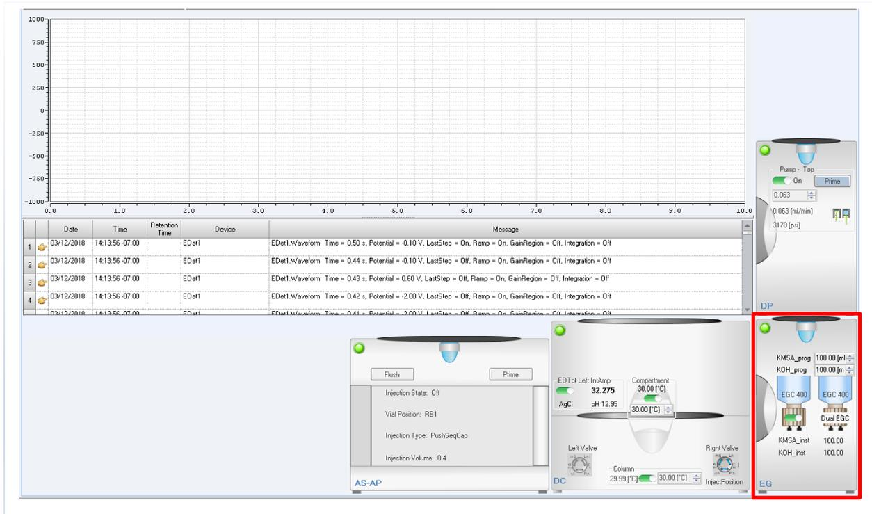
Figure 20 Chromeleon Console: Eluent Generator e-Panel of Dual EGC Mode
