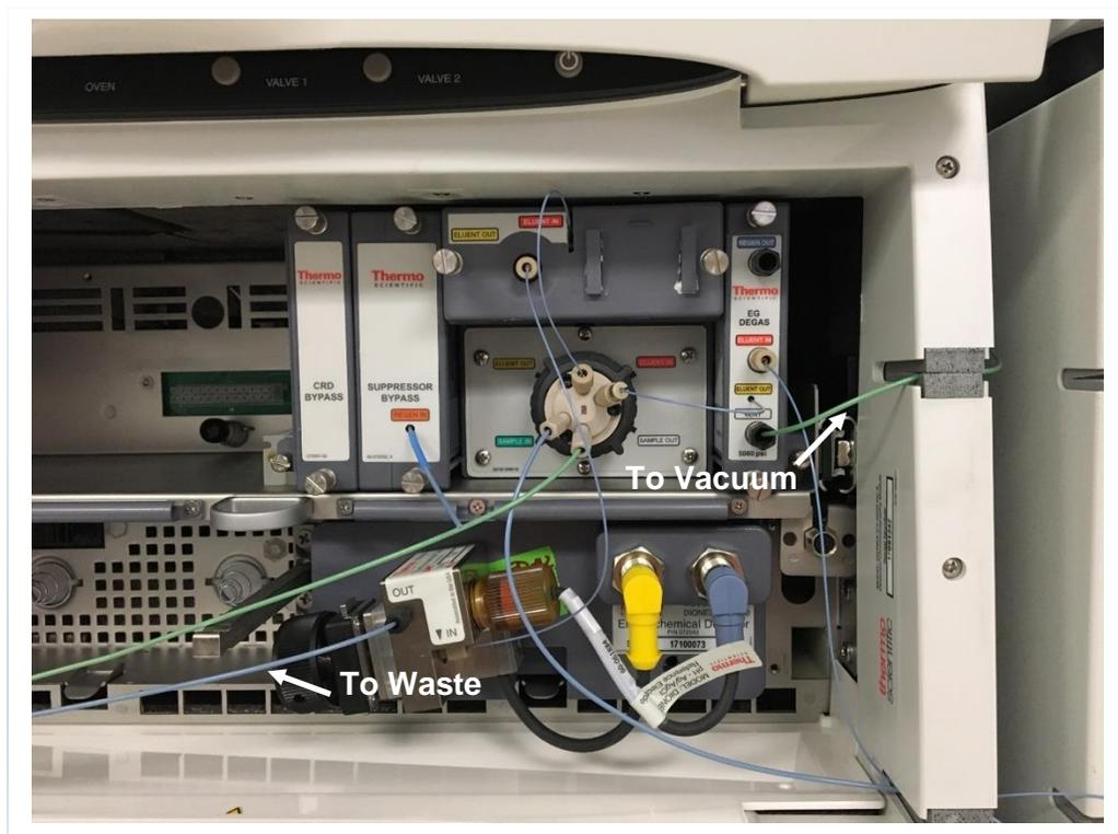
25. Connect the ELUENT OUT port of the Dionex Capillary RFIC Eluent Degasser (Item # 22181-60202) to a PEEK backpressure tubing (Item # 22181-20032). Direct the backpressure tubing to waste.
