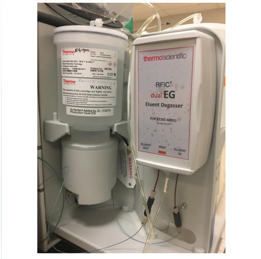
23. Direct the ELUENT OUT port of the Dionex RFIC<sup>+</sup> Dual EG Eluent Degasser (Item # 22181-60951) to waste.
