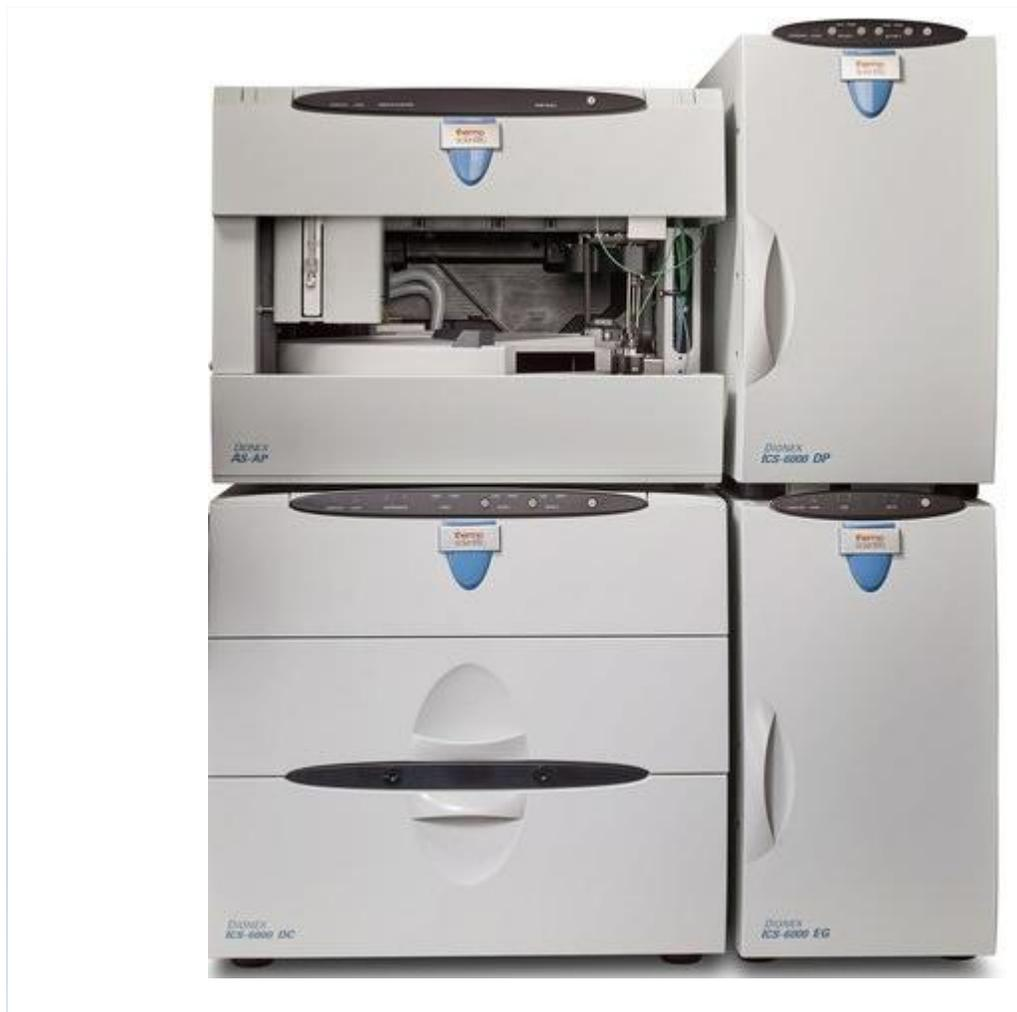
1. Fill a 2 L eluent reservoir bottle with ASTM filtered, Type I (18-megohm) degassed deionized water. Connect the reservoir to the eluent inlet line of the pump. Keep the water blanketed under an inert gas (helium or nitrogen).
