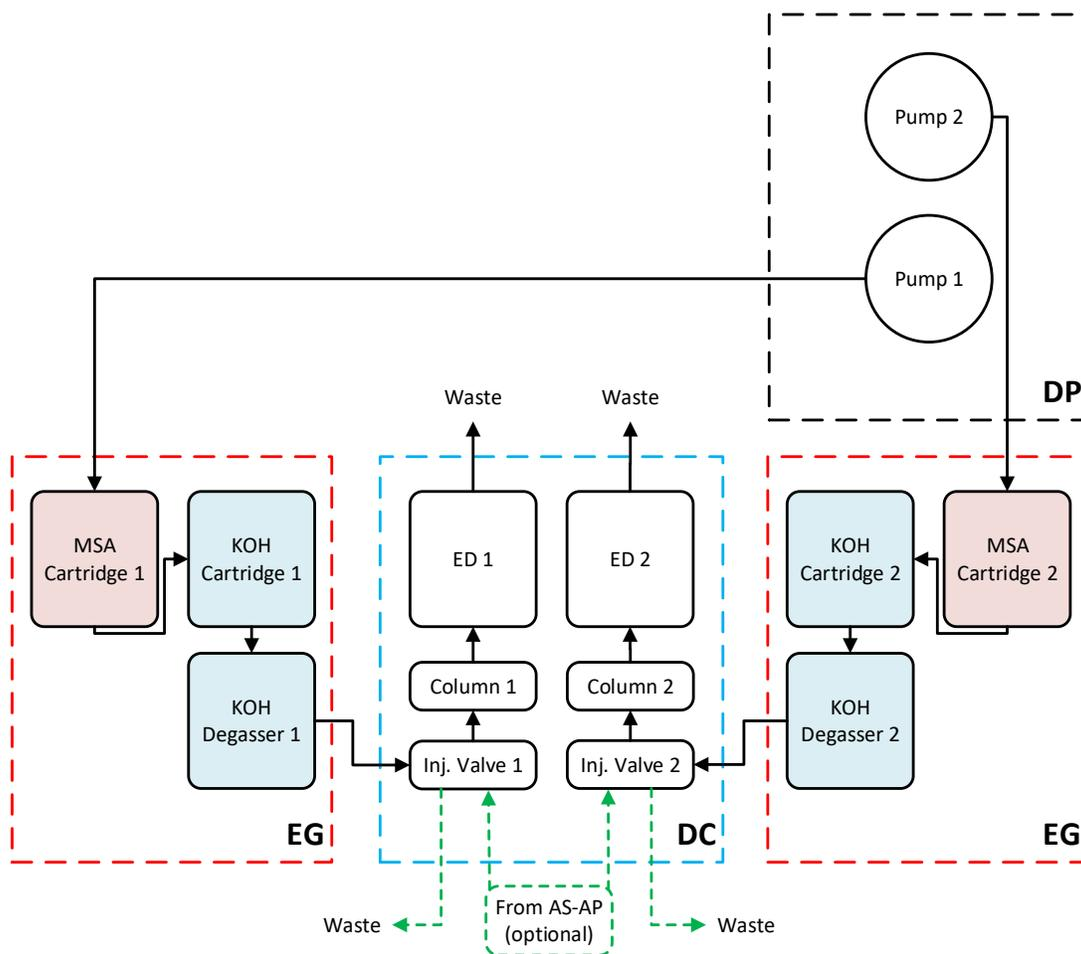
Figure 9 Dual Channel Hybrid Dual EGC Mode, Vacuum Connection
