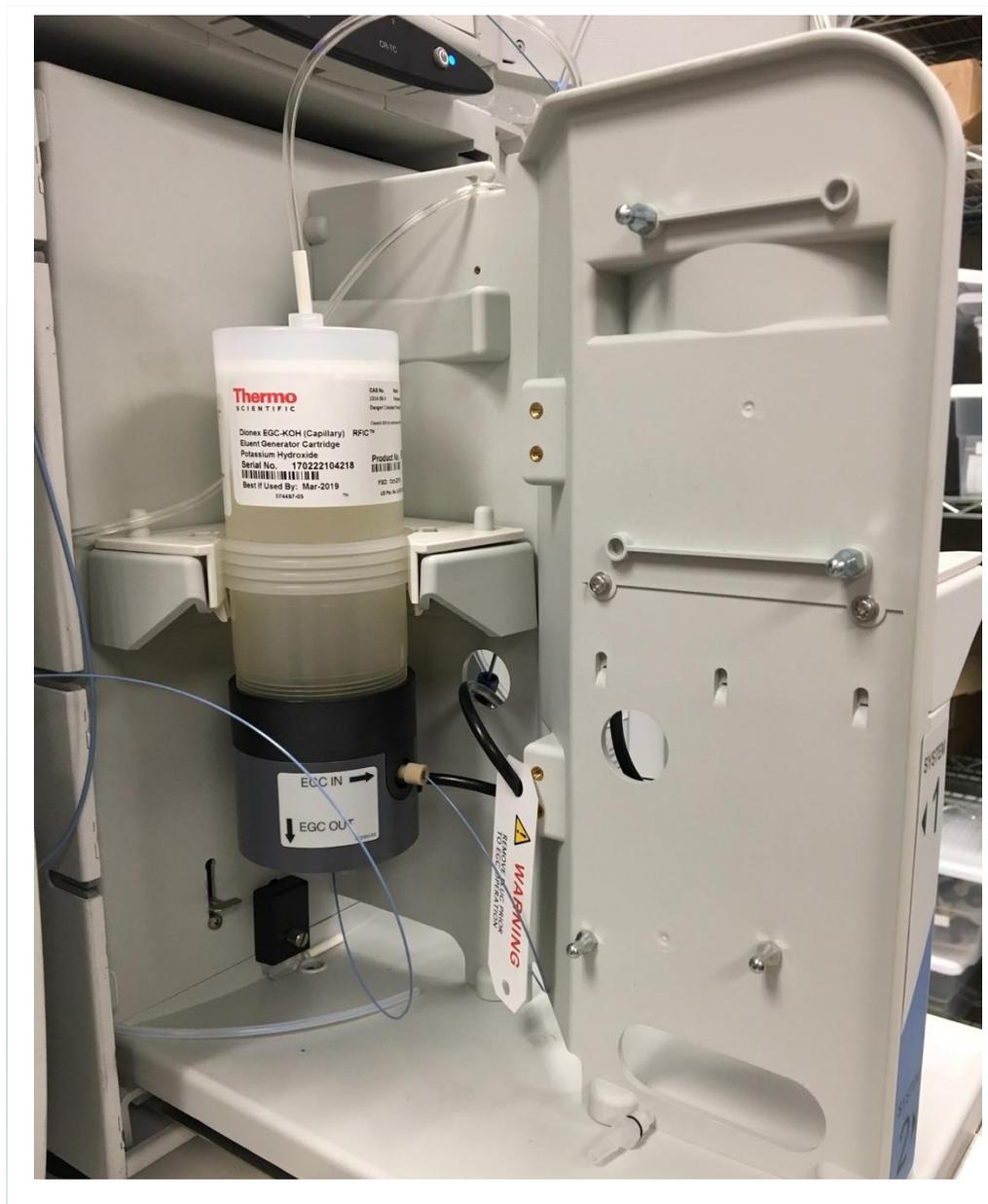
16. Turn on the pump and pump DI water through the Dionex EGC-KOH (Capillary) for 15 minutes at the flow rate of 0.1 mL/min.
