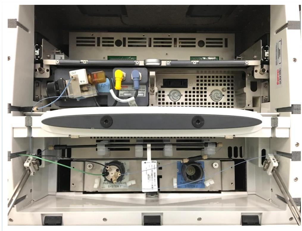
**Figure 6 View of DC Compartment, with Both the Guard and the Separator Column Installed.**
