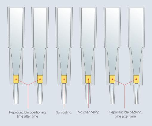
Figure 1: SOLAµ SPE design – limiting issues associated with conventional SPE formats
