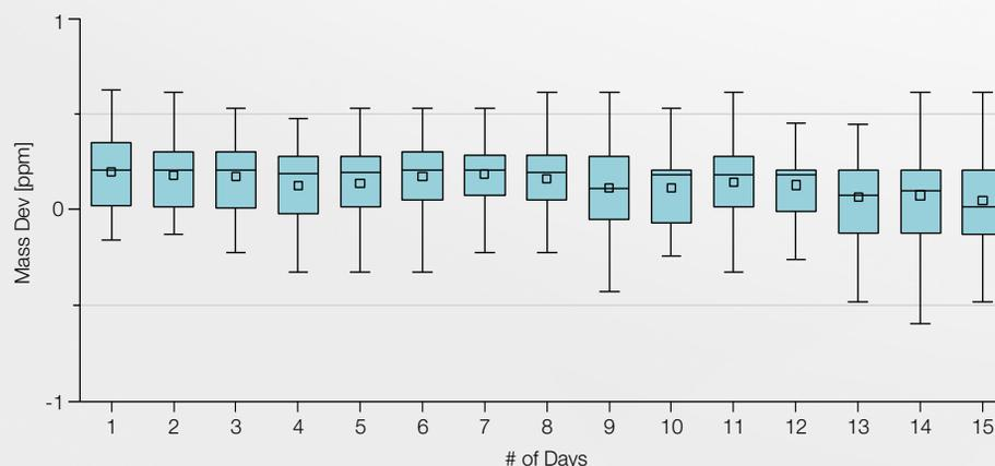
Through the use of Thermo Scientific EASY-IC ion source, sub-ppm mass accuracy is consistently delivered without user intervention for at least five days. A panel of veterinary drugs with  $m/z$  range from 160...900 was analyzed at 100  $\mu\text{g/L}$  over a 15 day period with continual polarity switching, providing exceptional mass accuracy.
