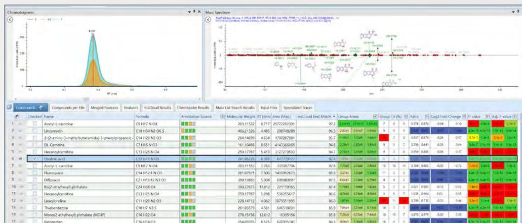
Unknown screening results shown with an integrated view in Compound Discoverer software, including raw data, chromatographic peak, and mass spectrum (including mirror plot with mzCloud match).
