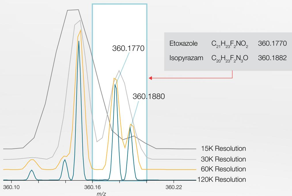
Full-scan mass spectrum of etoxazole and isopyrazam, measured using the Orbitrap Exploris 120 mass spectrometer at a resolution (R) setting up to 120,000 (FWHM) at  $m/z$  200, demonstrates outstanding resolving power.
