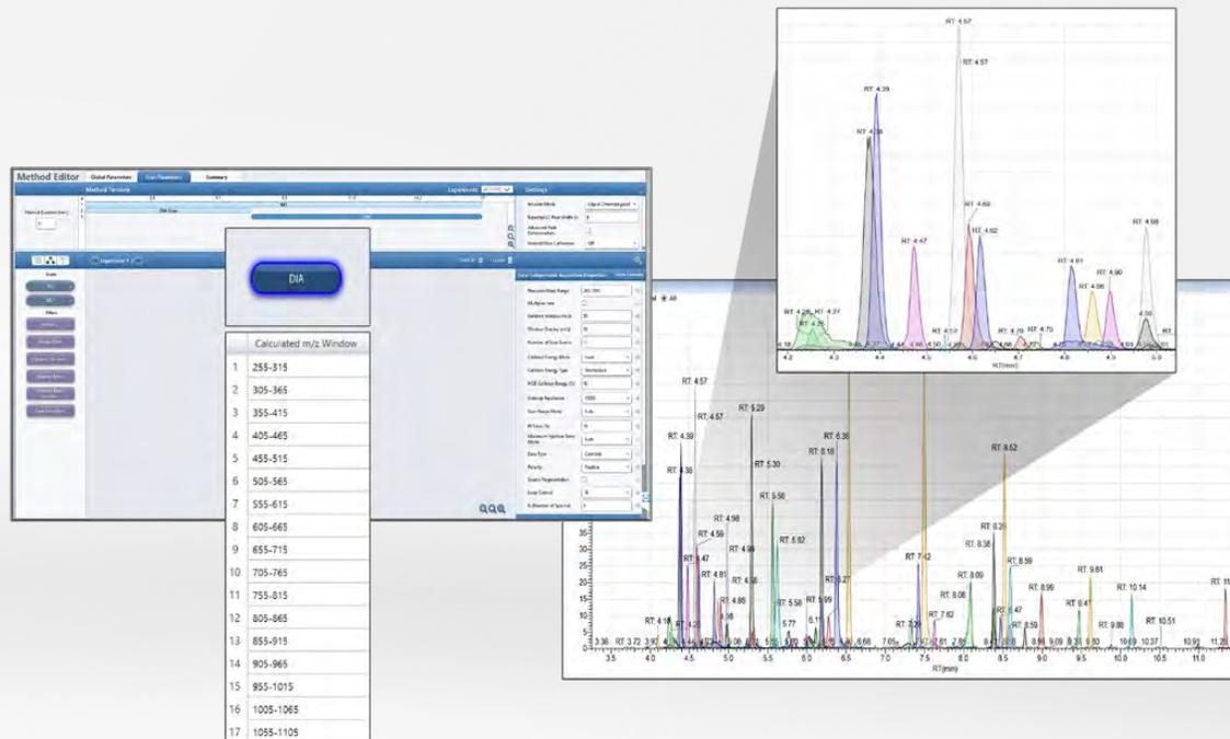
Quantitation of all compounds in bovine muscle matrix is easily achieved by fast scan speeds, even when multiple precursor ion  $m/z$  isolation windows are selected for the data-independent acquisition (DIA) experiment.
