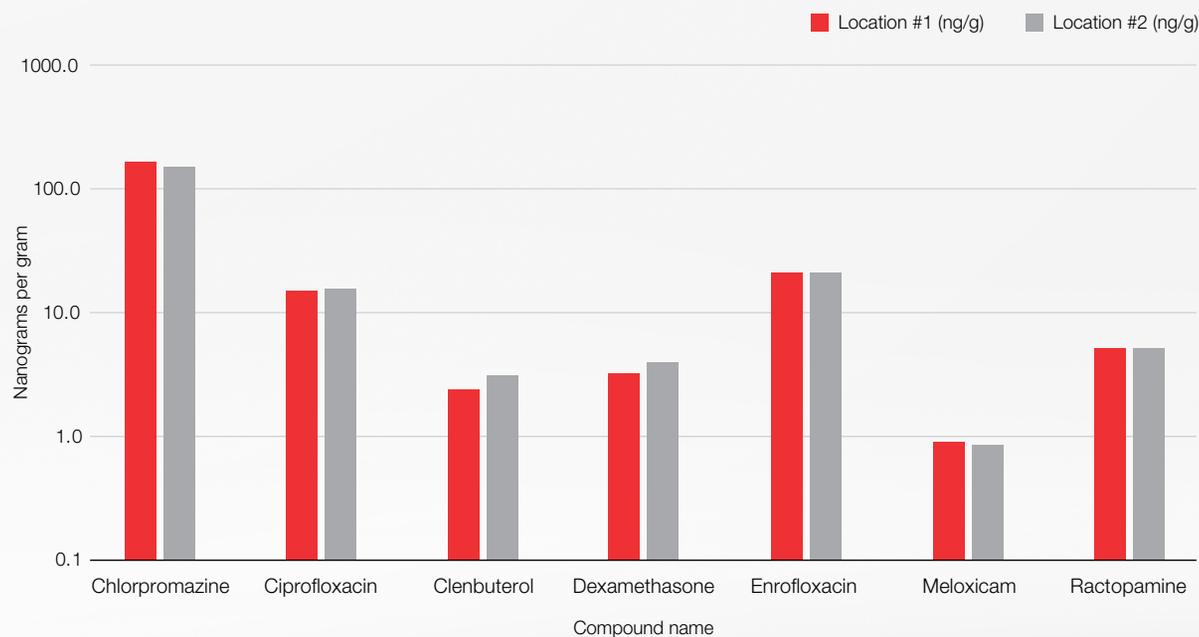
To assess LC-HRAM MS system-to-system reproducibility, two operators at two different locations analyzed the same sample of veterinary drug residues in bovine muscle matrix on two separate systems. The minimal 5.1% average difference observed in analyte concentrations demonstrate high reproducibility across multiple Orbitrap Exploris 120 mass spectrometer systems.
