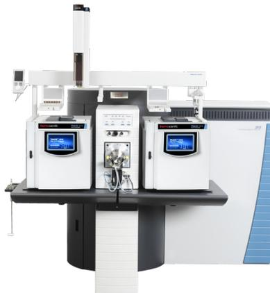
Unique double-GC configuration for maximum flexibility. For example PCDD/F on GC one and PCBs on GC two.
