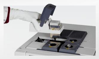
Access unprecedented flexibility. Switch instant-connect injectors and detectors in minutes without tools.
