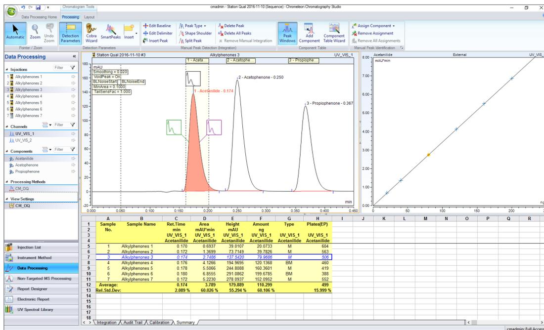
Figure 5. The Chromatography Studio provides easy and efficient access to all aspects of an injection sequence within a single window frame. The integrated design eliminates the need to launch and manage different windows when working with a data set allowing for fast, easy data review.
