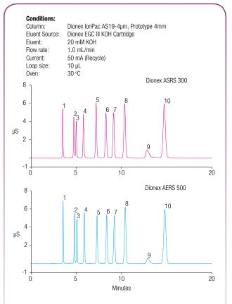
Figure 3: Comparison of the Dionex AERS 500 suppressor to the Dionex ASRS 300 suppressor using an inorganic anion standard. The Dionex AERS 500 suppressor outperforms the Dionex ASRS 300 suppressor, as shown by the peak efficiency and resolution
