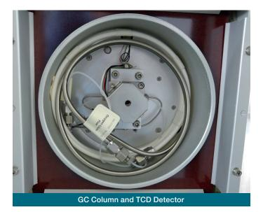
Figure 4. FlashSmart CHN and Oxygen internal circuits.
