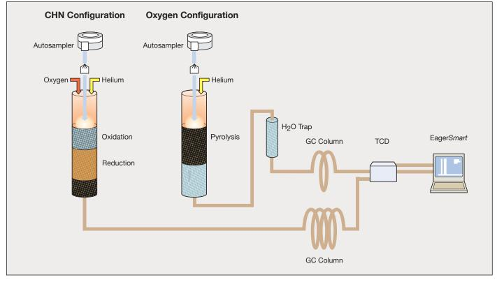
Figure 3. FlashSmart CHN/O configuration.
