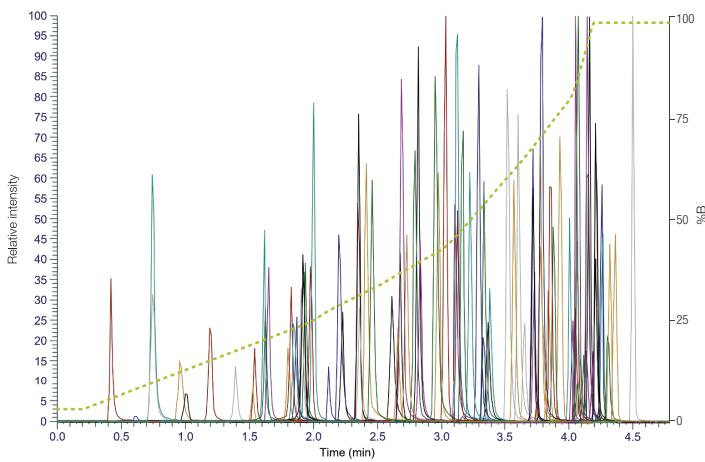
Figure 3. SRM chromatograms of 106 drugs of abuse with the mobile phase gradient overlaid
