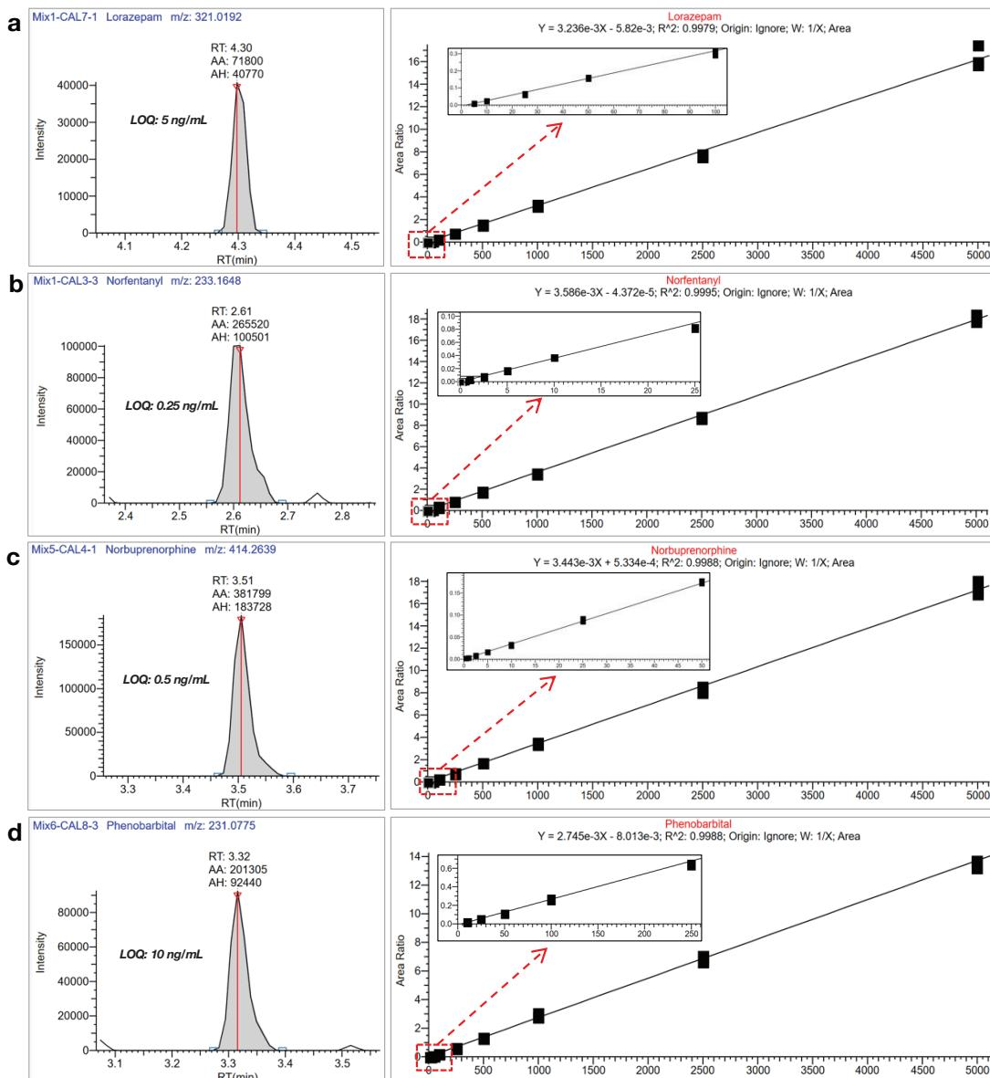
Figure 5. SRM chromatograms of (a) lorazepam, (b) norfentanyl, (c) norbuprenorphine, and (d) phenobarbital at their respective LOQ levels along with calibration curves
