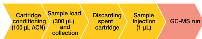
Figure 3. TriPlus RSH SMART extract clean-up and injection
