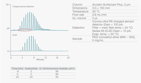
Figure 9. Sensitivity comparison of charged aerosol detection vs. ELSD
