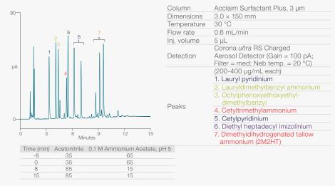
Figure 2. Separation of cationic surfactants
