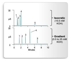
Figure 5: Chromatogram of water sample using isocratic versus gradient eluent concentrations.
