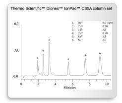
Figure 8: Chromatogram of various transition metals in water using Thermo Scientific™ Dionex™ IonPac™ CS5A column set.
