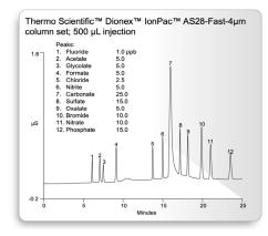
Figure 6: Achieving ppt-level determinations using Thermo Scientific™ Dionex™ IonPac™ AS28-Fast-4µm column set (500 µL injection)
