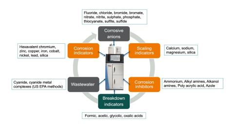
Figure 11: Example analyses performed by Thermo Scientific<sup>™</sup> Dionex<sup>™</sup> ion chromatography systems.
