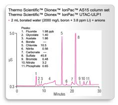
Figure 9: Chromatogram of trace ions in water containing higher concentrations of boron and lithium.
