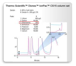
Figure 7: Detecting small concentrations of corrosion inhibitors in the presence of larger signals.
