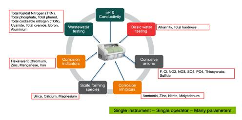
Figure 10: Example analyses performed by the Thermo Scientific™ Gallery™ Plus Discrete Analyzer.
