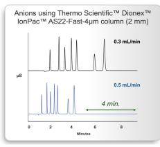
Figure 4: Impact of increasing flow rate through the Thermo Scientific<sup>™</sup> Dionex<sup>™</sup> IonPac<sup>™</sup> AS22-Fast-4µm column (2 mm) on the chromatogram of inorganic anions.
