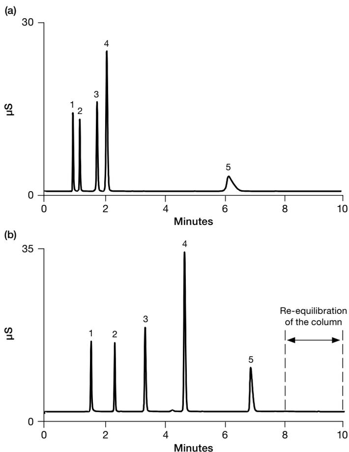
**Figure 1. Separation of inorganic anions with an electrolytically generated KOH eluent.** Separator column: Dionex IonPac AS11; column format: 250 mm  $\times$  4 mm i.d.; eluent: (a) 15.5 mmol/L KOH, (b) 0.5–25 mmol/L KOH in 8 min; flow rate: 2 mL/min; detection: suppressed conductivity; injection volume: 25  $\mu$ L; peaks: 2 mg/L fluoride (1), 3 mg/L chloride (2), 10 mg/L nitrate (3), 15 mg/L sulfate (4), and 15 mg/L orthophosphate (5).
