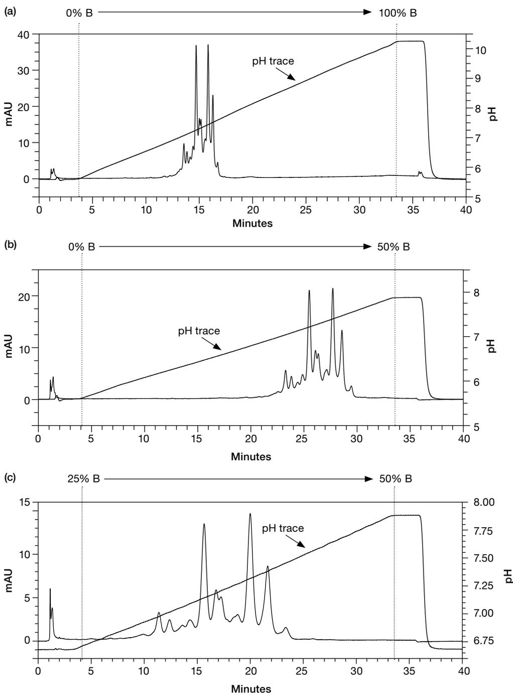
**Figure 13. Optimization of the separation of mAb charge variants with a linear pH gradient.** Separator column: Dionex MAbPac SCX-10, 10  $\mu$ m; column format: 250 mm  $\times$  4 mm i.d.; eluent: pH gradient based on the CX-1 buffer system; gradient: (a) 0% B (pH 5.6) to 100% B (pH 10.2) in 30 min, (b) 0% B (pH 5.6) to 50% B (pH 7.9), (c) 25% B (pH 6.75) to 50% B (pH 7.9).
