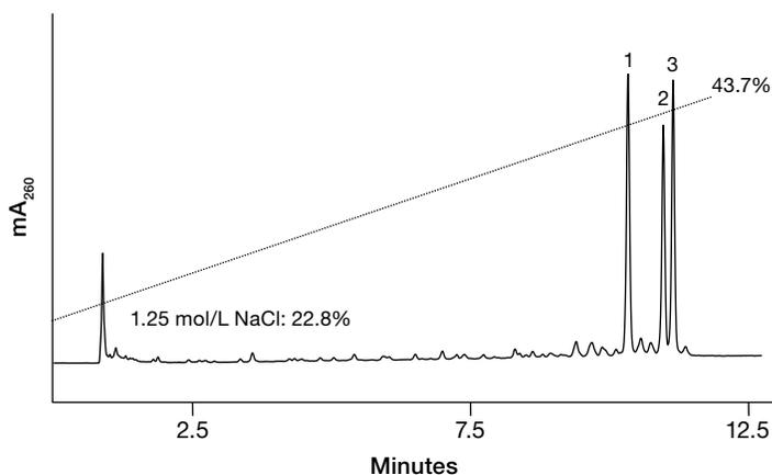
**Figure 8. Gradient elution of an oligonucleotide mixture such as d(AC)<sub>10–11</sub> 20–22-mers.** Separator column: Dionex DNAPac PA200; column format: 250 mm × 4 mm i.d.; column temperature: 25 °C; eluent: (A) 20 mmol/L Tris (pH 8), (B) 20 mmol/L Tris + 1.25 mol/L NaCl (pH 8); gradient: linear from 22.8% B to 43.7% B in 12 min; flow rate: 1.2 mL/min; detection: UV (268 nm); injection volume: 8 µL; peaks: (1) 20-mer, (2) 21-mer, and (3) 22-mer.
