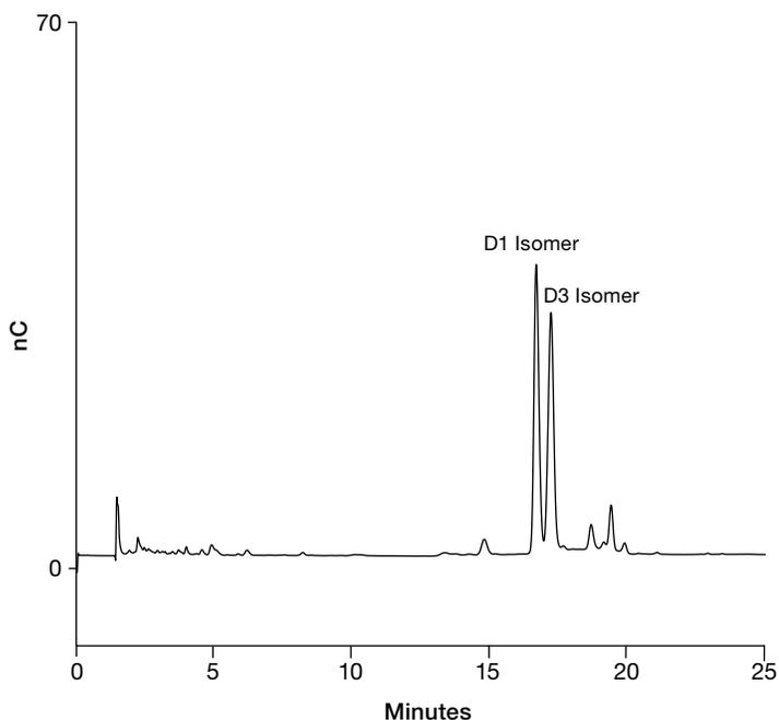
**Figure 6. Gradient elution of mannose-7 linkage isomers.** Separator column: Dionex CarboPac PA200; column format: 250 mm × 3 mm i.d.; eluent: NaOH/NaOAc; gradient: 0–200 mmol/L NaOAc in 100 mmol/L NaOH in 110 min; flow rate: 0.5 mL/min; detection: integrated pulsed amperometry on a gold working electrode; sample: mannose-7 linkage isomers (Dextra Labs, Reading, UK).
