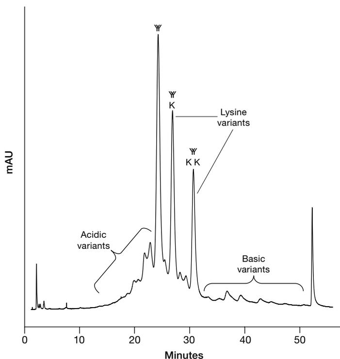
**Figure 12. Gradient elution of a monoclonal antibody with a MES/NaCl eluent.** Separator column: Dionex MAbPac SCX-10, 10  $\mu$ m; column format: 250 mm  $\times$  4 mm i.d.; column temperature: 30  $^{\circ}$ C; eluent: A. 20 mmol/L MES + 60 mmol/L NaCl, pH 5.6, B. 20 mmol/L MES + 300 mmol/L NaCl, pH 5.6; gradient: 15–36.44% in 50 min; flow rate: 1 mL/min; detection: UV (280 nm); injection volume: 10  $\mu$ L; sample: 5 mg/mL mAb.
