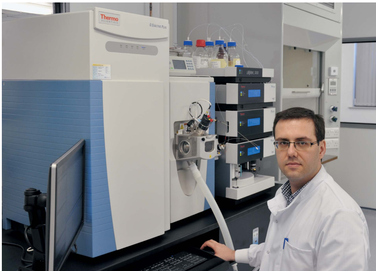
▲ NCFS scientist, Dr. Lukas Vaclavik, performs an analysis on a Q Exactive Plus mass spectrometer in a Covance laboratory in Harrogate, UK.
