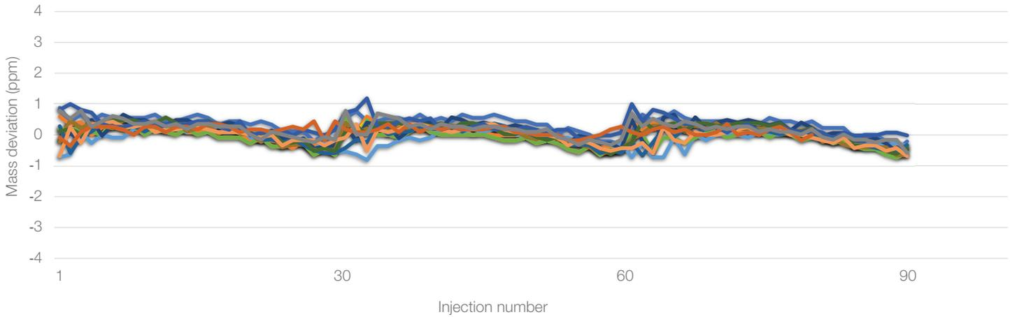
**Figure 3. Mass accuracy for 90 calibration and quality control standards injected over three days of analysis.** % RSD for all repeated injected standards was < 0.5%.
