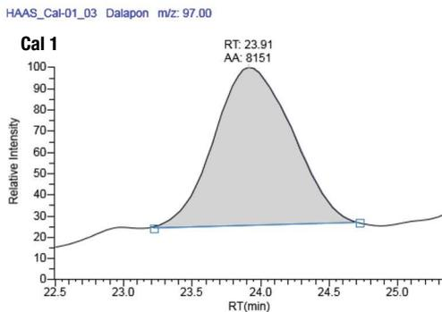
Figure 3-3. Calibration curve with the chromatogram at the lowest concentration calibrator (0.25 µg/L) for each HAA: (H) DBCAA, (I) BDCAA, (J) Bromate, and (K) Dalapon
