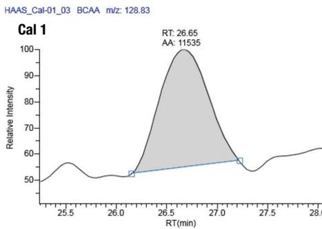
Figure 3-2. Calibration curve with the chromatogram at the lowest concentration calibrator (0.25 µg/L) for each HAA: (D) DBAA, (E) TCAA, (F) TBAA, (G) BCAA
