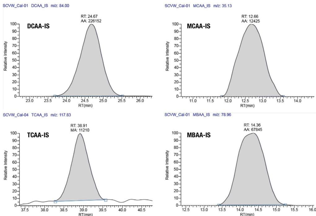
Figure 2. Ion chromatograms of the internal standards of the four mentioned analytes at 4  $\mu\text{g/L}$
