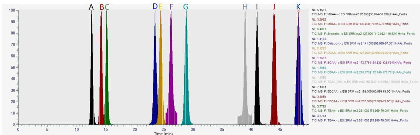
Figure 1. Ion chromatograms of HAAs: (A) MCAA, (B) MBAA, (C) Bromate, (D) Dalapon, (E) DCAA, (F) BCAA, (G) DBAA, (H) TCAA, (I) BDCAA, (J) DBCAA and (K) TBAA at 1  $\mu\text{g/L}$
