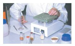
Figure 5. Kit for Total Organic Carbon (TOC) for solid samples.
