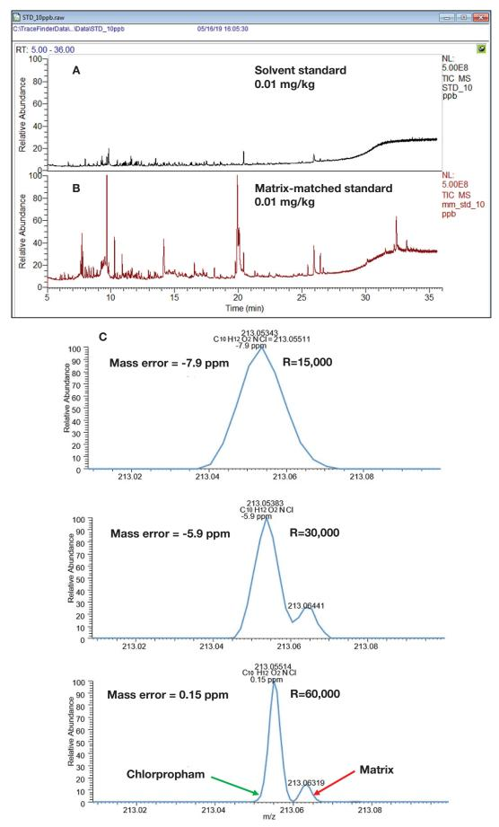
Figure 1. Comparison of total ion chromatogram for solvent standard (A) and matrix-matched standard (B), and the impact of resolving power on chlorpropham ( $C_{10}H_{12}CINO_2$  theoretical mass *m/z* 213.055116) selectivity at various resolving power settings of 15,000, 30,000, and 60,000 (C)
