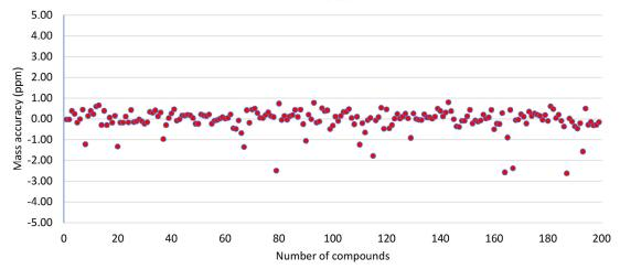
Figure 4. Observed average mass accuracy for all 197 molecules in n=35 replicates of a 0.025 mg/kg pre-spiked potato sample.
