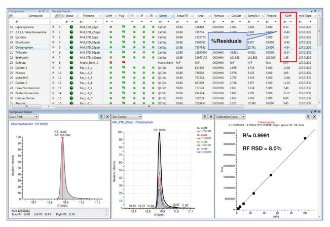
Figure 3. Screening and quantification of chlorpropham based on confirmation criteria
